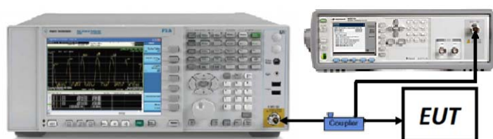
Figure 7-3. Test Instrument & Measurement Setup
