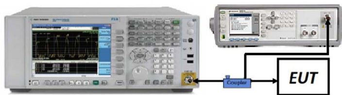
Figure 7-4. Test Instrument & Measurement Setup
