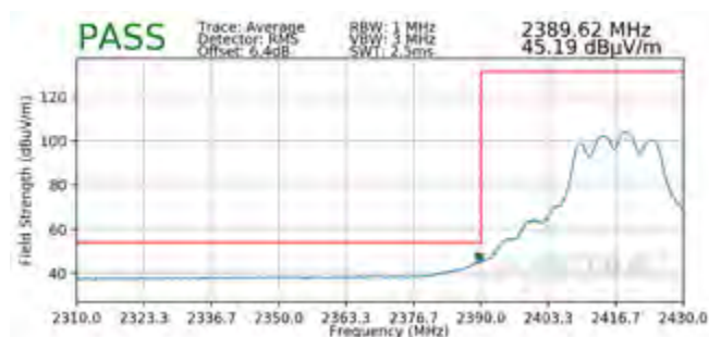
Plot 7-111. Radiated Restricted Lower Band Edge Measurement CDD (Average)
