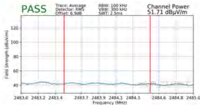
Plot 7-103. Radiated Restricted Upper Band Edge Measurement SISO ANT2 (Average)
