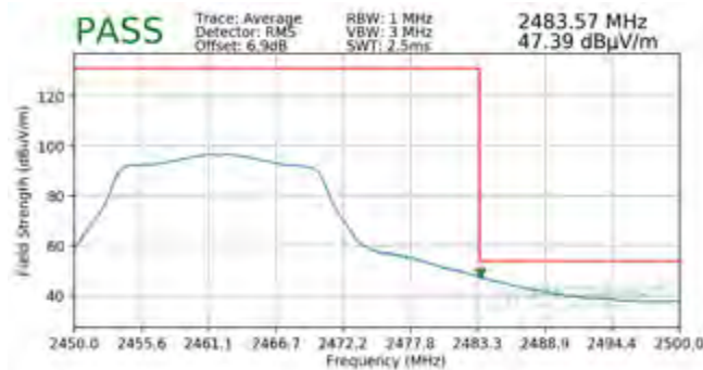
Plot 7-101. Radiated Restricted Upper Band Edge Measurement SISO ANT2 (Average)
