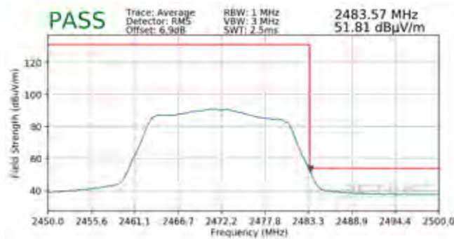
Plot 7-135. Radiated Restricted Band Edge Measurement MIMO with WCP (Average)
