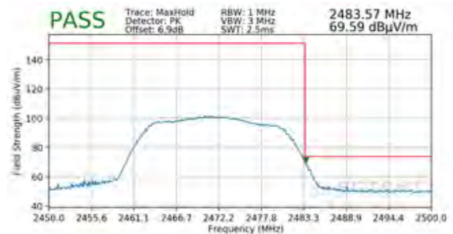
Plot 7-136. Radiated Restricted Band Edge Measurement MIMO with WCP (Peak)
