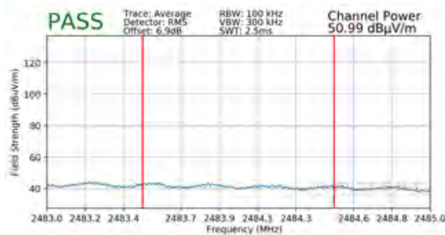
Plot 7-119. Radiated Restricted Upper Band Edge Measurement CDD (Average)
