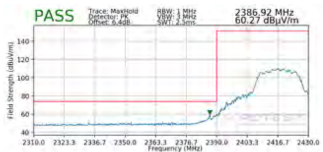
Plot 7-126. Radiated Restricted Lower Band Edge Measurement MIMO (Peak)
