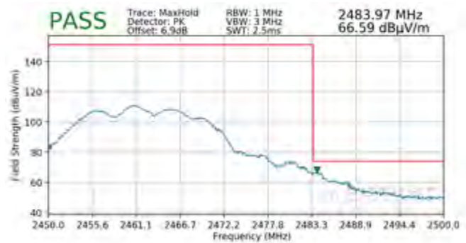
Plot 7-122. Radiated Restricted Band Edge Measurement CDD with WCP (Peak)
