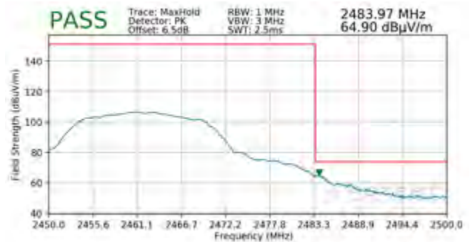
Plot 7-88. Radiated Restricted Upper Band Edge Measurement SISO ANT1 (Peak)
