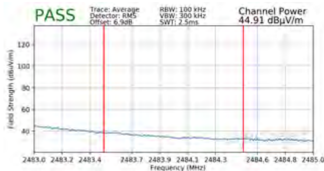
Plot 7-133. Radiated Restricted Upper Band Edge Measurement MIMO (Average)
