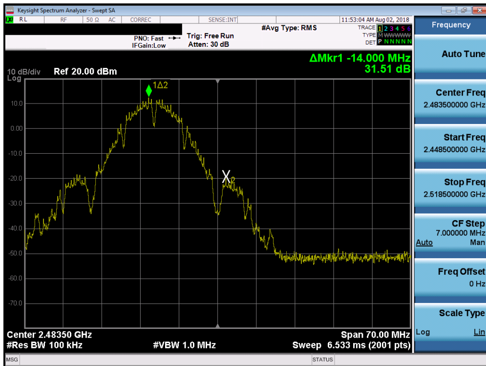
Plot 7-40. Band Edge Plot SISO ANT1 (802.11b – Ch. 13)
