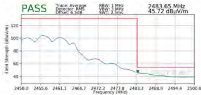
Plot 7-113. Radiated Restricted Upper Band Edge Measurement CDD (Average)
