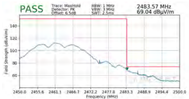
Plot 7-116. Radiated Restricted Upper Band Edge Measurement CDD (Peak)
