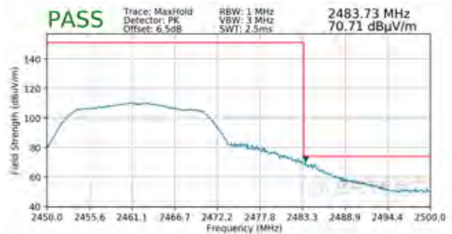
Plot 7-130. Radiated Restricted Upper Band Edge Measurement MIMO (Peak)
