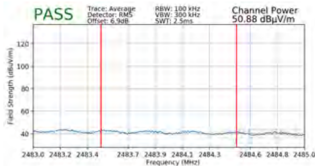
Plot 7-131. Radiated Restricted Upper Band Edge Measurement MIMO (Average)
