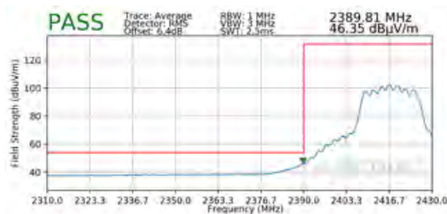
Plot 7-125. Radiated Restricted Lower Band Edge Measurement MIMO (Average)
