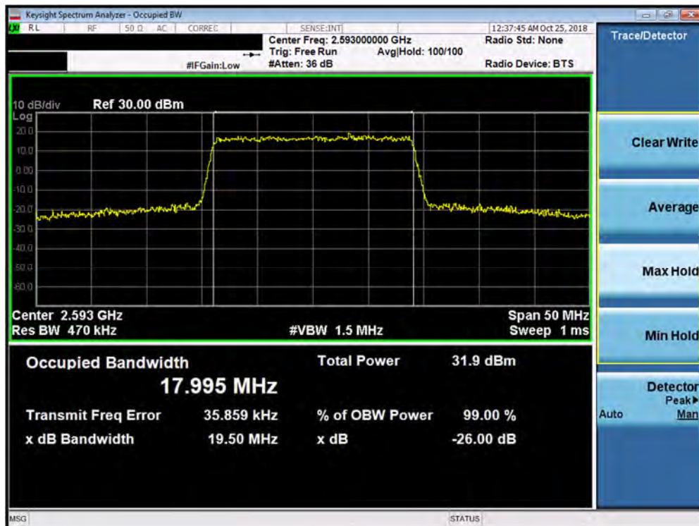
Plot 7-40. Occupied Bandwidth Plot (Band 41 - 20.0MHz QPSK - Full RB Configuration)
