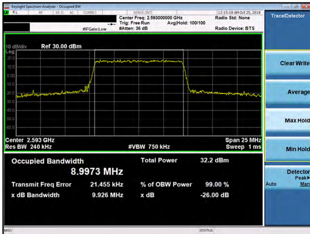
Plot 7-34. Occupied Bandwidth Plot (Band 41 - 10.0MHz QPSK - Full RB Configuration)
