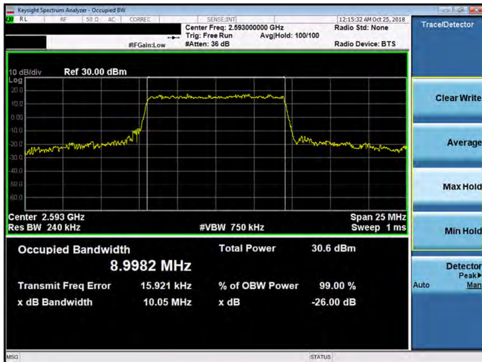
Plot 7-36. Occupied Bandwidth Plot (Band 41 - 10.0MHz 64-QAM - Full RB Configuration)
