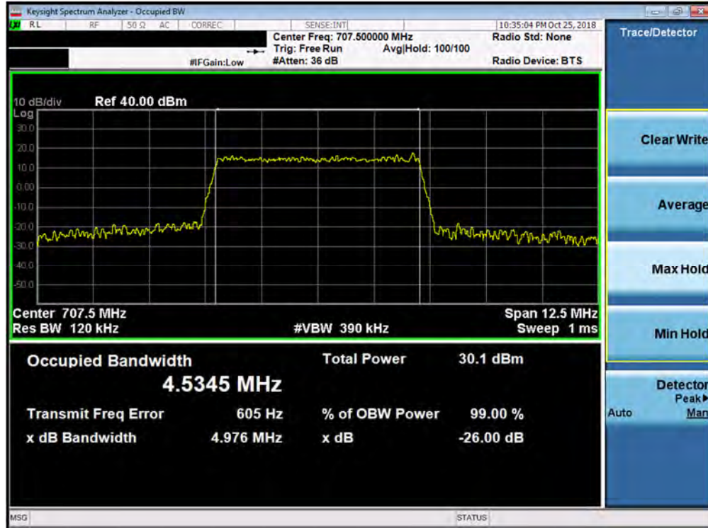
Plot 7-9. Occupied Bandwidth Plot (Band 12 - 5.0MHz 64-QAM - Full RB Configuration)
