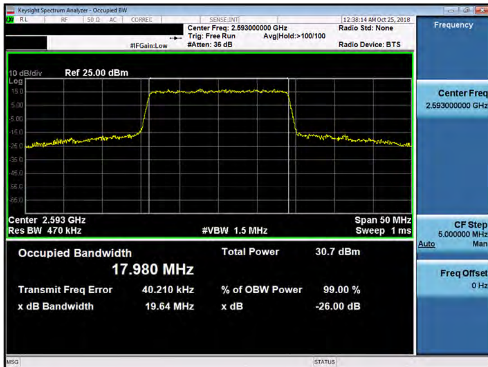
Plot 7-42. Occupied Bandwidth Plot (Band 41 - 20.0MHz 64-QAM - Full RB Configuration)
