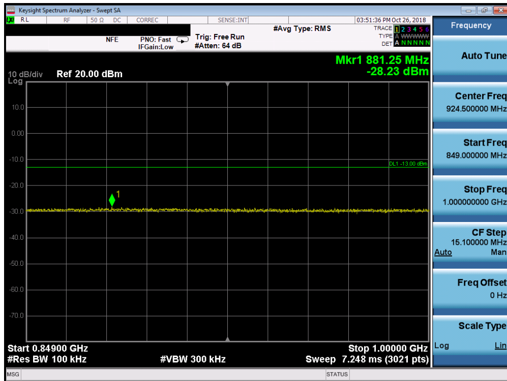
Plot 7-25. Conducted Spurious Plot (Cellular WCDMA Mode - Low Channel)
