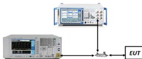
Figure 7-1. Test Instrument & Measurement Setup
