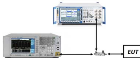
Figure 7-3. Test Instrument & Measurement Setup
