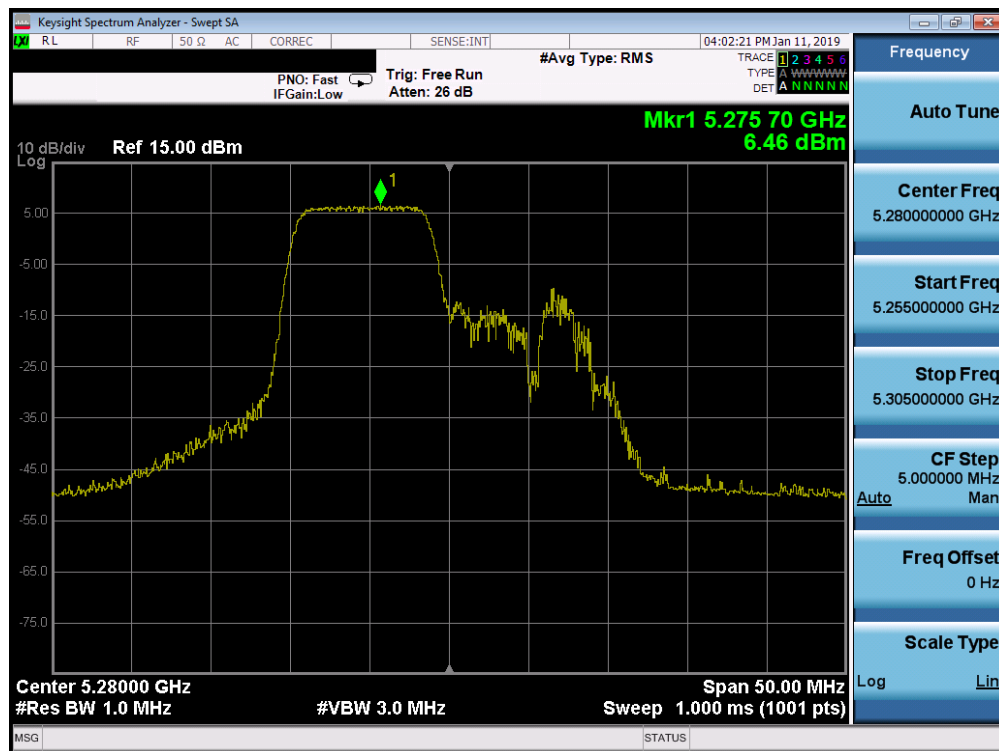
Plot 7-299. Power Spectral Density Plot SISO ANT2 (20MHz BW 802.11ax – 106 Tones (UNII Band 2A) – Ch. 56)
