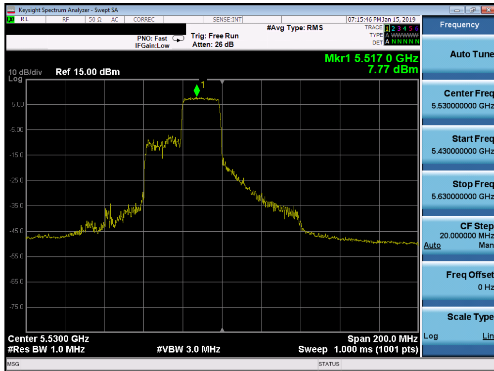
Plot 7-337. Power Spectral Density Plot SISO ANT2 (80MHz BW 802.11ax – 242 Tones (UNII Band 2C) – Ch. 106)
