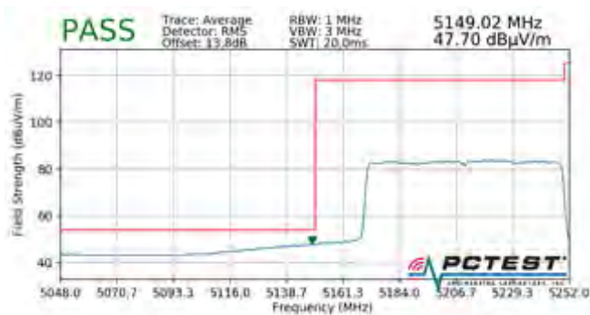
Plot 7-748. Radiated Lower Band Edge Plot SISO ANT2 (Average – UNII Band 1 – 996 Tones)
