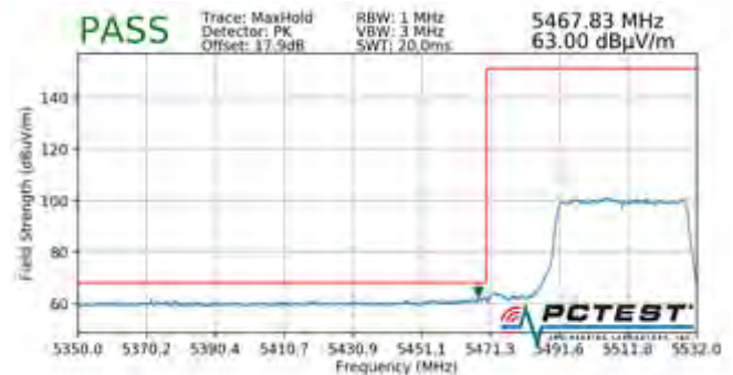
Plot 7-785. Radiated Lower Band Edge Plot MIMO (Peak – UNII Band 2C – 484 Tones)
