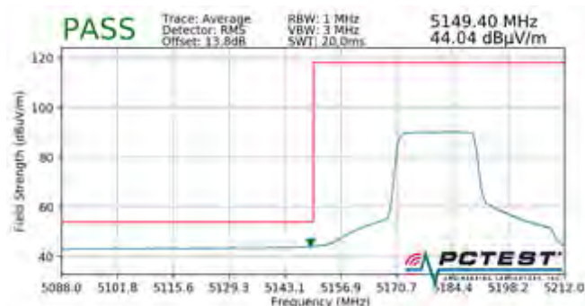
Plot 7-725. Radiated Lower Band Edge Plot SISO ANT2 (Average – UNII Band 1 – 242 Tones)
