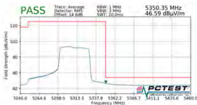
Plot 7-695. Radiated Upper Band Edge Plot SISO ANT1 (Average - UNII Band 2A - 484 Tones)
