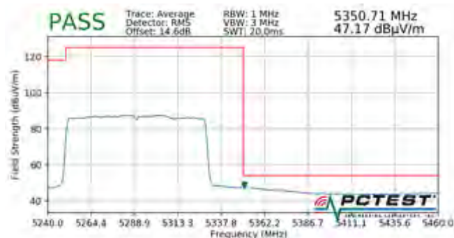
Plot 7-702. Radiated Upper Band Edge Plot SISO ANT1 (Average - UNII Band 2A - 996 Tones)
