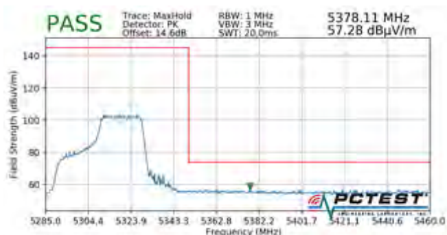
Plot 7-728. Radiated Upper Band Edge Plot SISO ANT2 (Peak – UNII Band 2A – 242 Tones)
