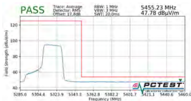
Plot 7-775. Radiated Upper Band Edge Plot MIMO (Average – UNII Band 2A – 242 Tones)
