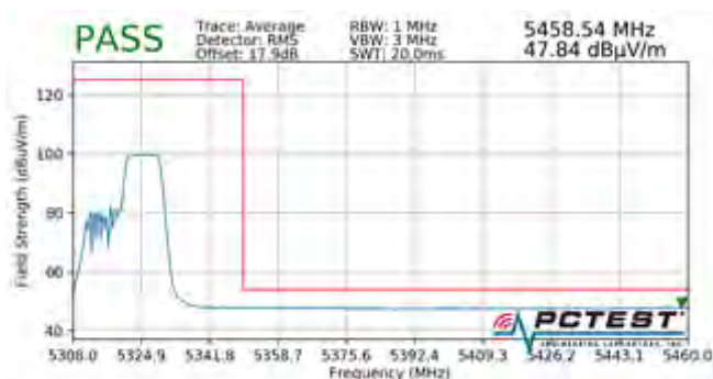
Plot 7-759. Radiated Upper Band Edge Plot MIMO (Average – UNII Band 2A – 106 Tones)
