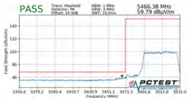
Plot 7-689. Radiated Lower Band Edge Plot SISO ANT1 (Peak – UNII Band 2C – 484 Tones)
