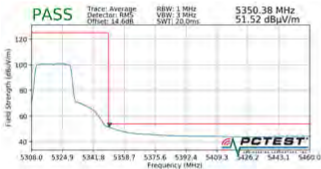
Plot 7-670. Radiated Upper Band Edge Plot SISO ANT1 (Average – UNII Band 2A – 242 Tones)
