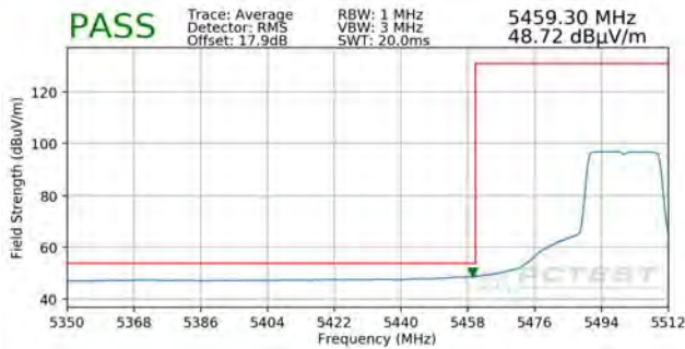
Plot 7-723. Radiated Band Edge Plot SISO ANT2 (Average – WCP – 242 Tones)
