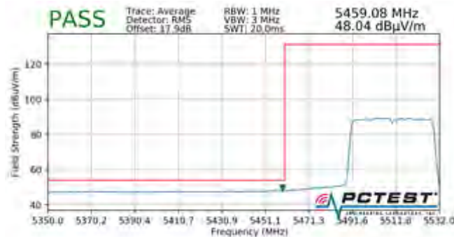
Plot 7-784. Radiated Lower Band Edge Plot MIMO (Average – UNII Band 2C – 484 Tones)
