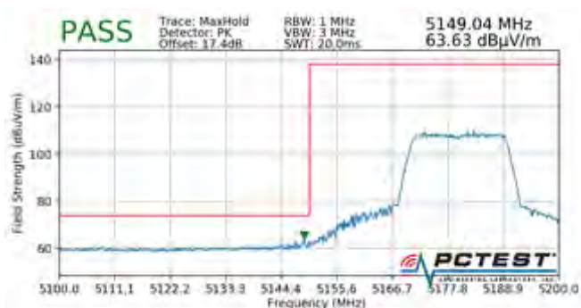
Plot 7-765. Radiated Lower Band Edge Plot MIMO (Peak – UNII Band 1 – 242 Tones)
