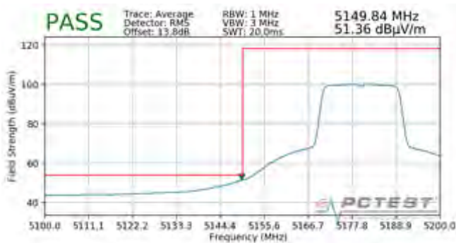
Plot 7-668. Radiated Lower Band Edge Plot SISO ANT1 (Average – UNII Band 1 – 242 Tones)
