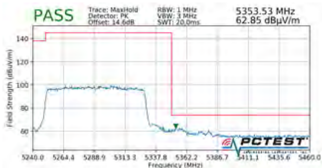
Plot 7-703. Radiated Upper Band Edge Plot SISO ANT1 (Peak - UNII Band 2A - 996 Tones)
