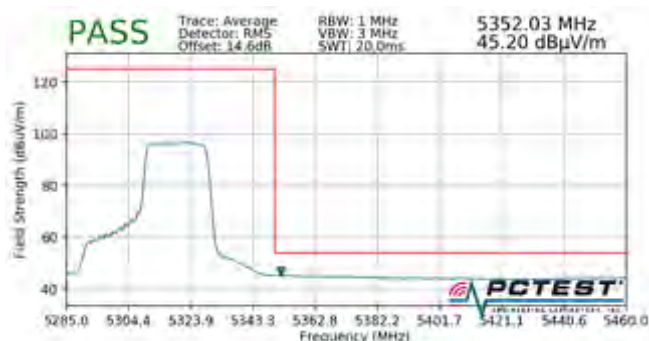
Plot 7-679. Radiated Upper Band Edge Plot SISO ANT1 (Average – UNII Band 2A – 242 Tones)
