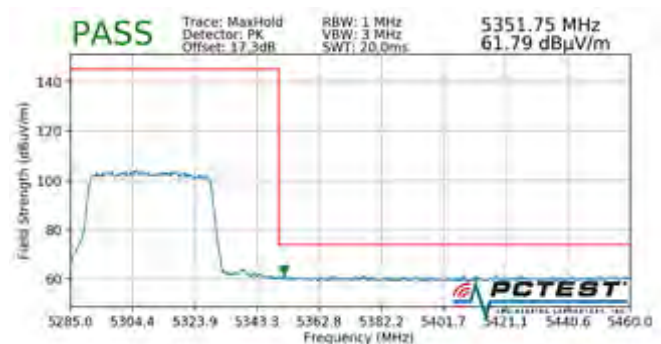
Plot 7-783. Radiated Upper Band Edge Plot MIMO (Peak – UNII Band 2A – 484 Tones)
