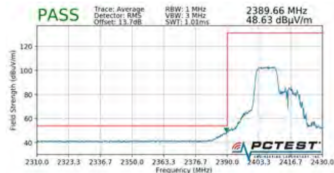
Plot 7-189. Radiated Restricted Lower Band Edge Measurement MIMO (Average – 106 Tones)
