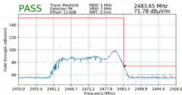
Plot 7-160. Radiated Restricted Upper Band Edge Measurement SISO ANT1 (Peak – 26 Tones)
