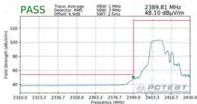
Plot 7-153. Radiated Restricted Lower Band Edge Measurement SISO ANT1 (Average – 106 Tones)
