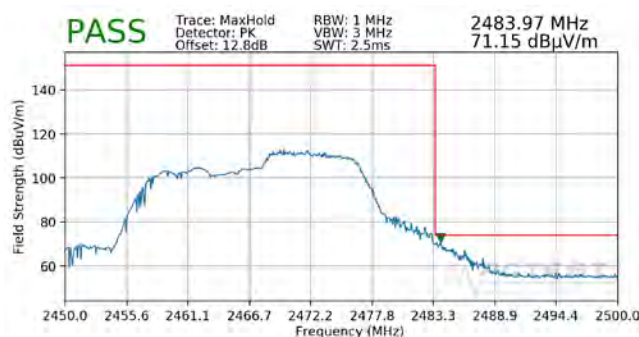
Plot 7-176. Radiated Restricted Upper Band Edge Measurement SISO ANT1 (Peak - 106 Tones)
