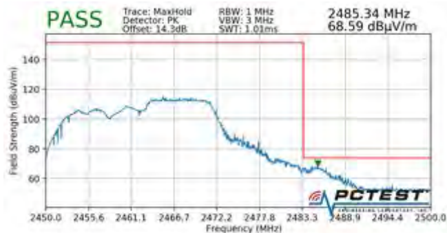
Plot 7-192. Radiated Restricted Upper Band Edge Measurement MIMO (Peak – 106 Tones)
