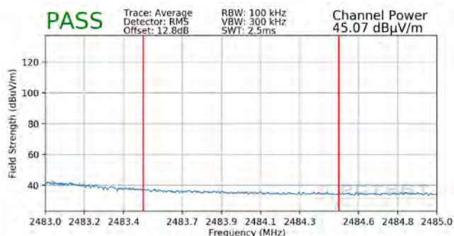
Plot 7-195. Radiated Restricted Upper Band Edge Measurement MIMO (Average - 106 Tones)
