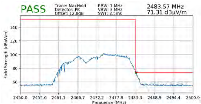
Plot 7-196. Radiated Restricted Upper Band Edge Measurement MIMO (Peak - 106 Tones)
