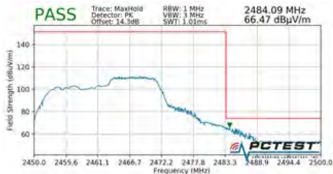
Plot 7-174. Radiated Restricted Upper Band Edge Measurement SISO ANT2 (Peak – 106 Tones)
