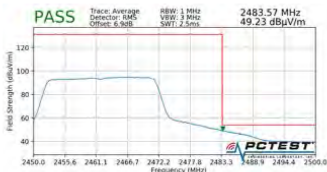
Plot 7-199. Radiated Restricted Upper Band Edge Measurement MIMO (Average - 242 Tones)
