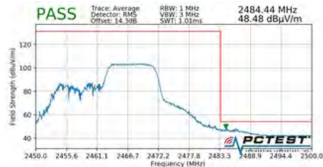
Plot 7-191. Radiated Restricted Upper Band Edge Measurement MIMO (Average – 106 Tones)
