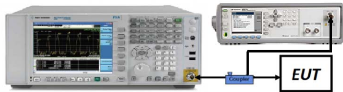
Figure 7-7. Test Instrument & Measurement Setup
