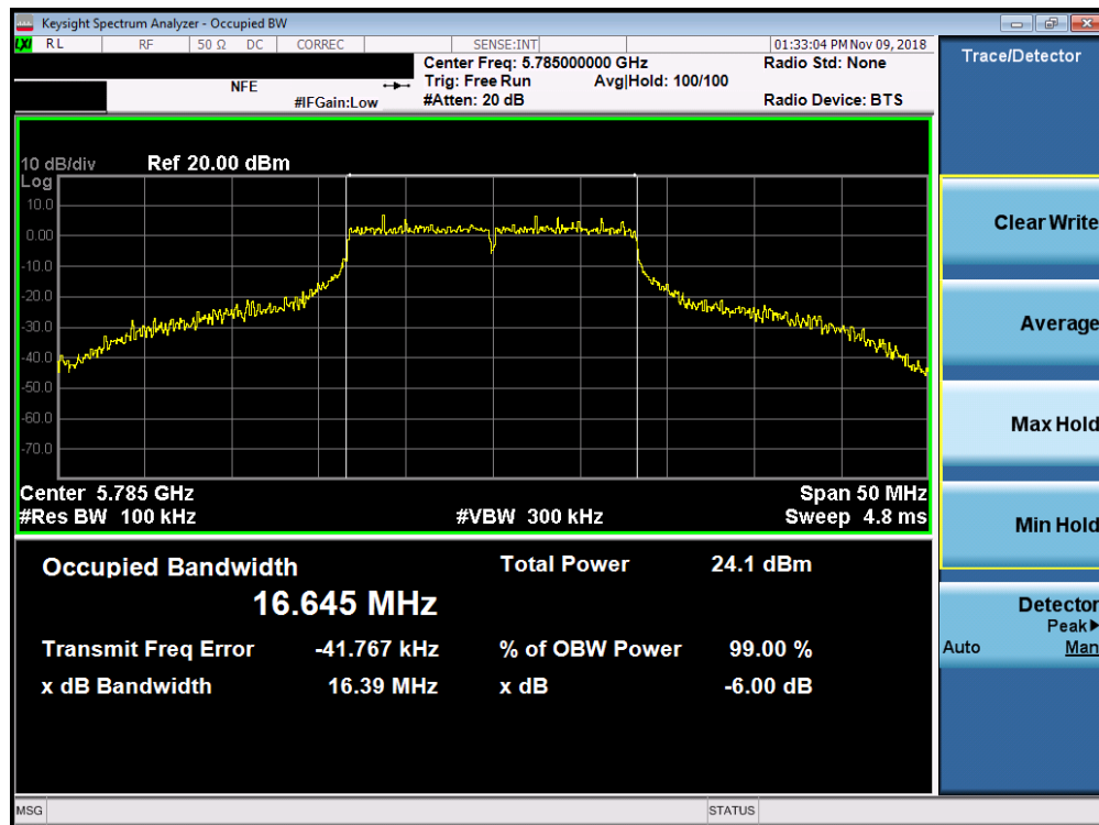
Plot 7-104. 6dB Bandwidth Plot SISO ANT1 (802.11a (UNII Band 3) – Ch. 157)
