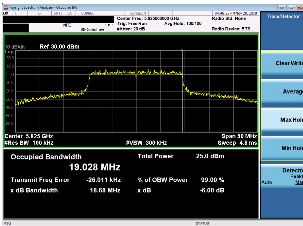
Plot 7-111. 6dB Bandwidth Plot SISO ANT1 (20MHz BW 802.11ax (UNII Band 3) – Ch. 165)
