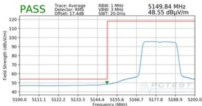
Plot 7-319. Radiated Lower Band Edge Plot SISO ANT2 (Average – UNII Band 1)
