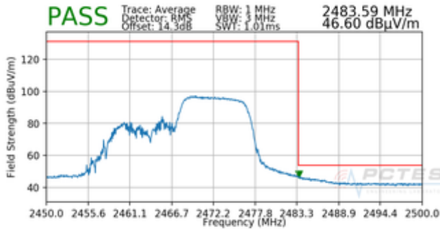
Plot 7-209. Radiated Restricted Upper Band Edge Measurement MIMO (Average – 106 Tones)
