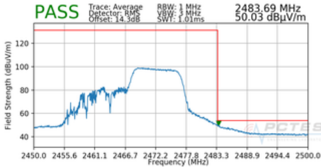
Plot 7-165. Radiated Restricted Upper Band Edge Measurement SISO ANT1 (Average – 106 Tones)
