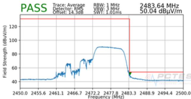
Plot 7-189. Radiated Restricted Upper Band Edge Measurement SISO ANT2 (Average – 242 Tones)
