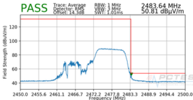
Plot 7-167. Radiated Restricted Upper Band Edge Measurement SISO ANT1 (Average – 106 Tones)
