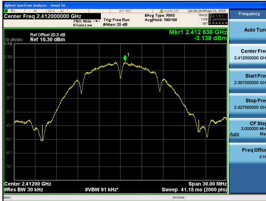
Power Spectral Density (802.11b-CH 1)
