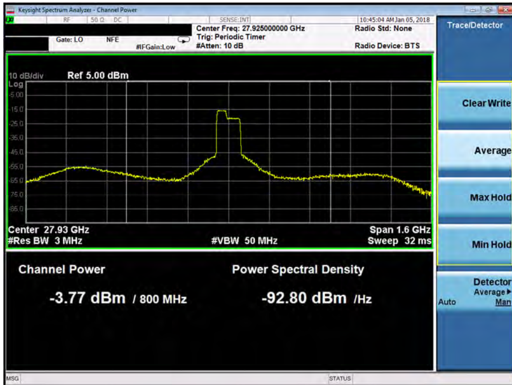
Plot 7-155. Antenna D EIRP Plot (1CC 16QAM Mid Channel)
