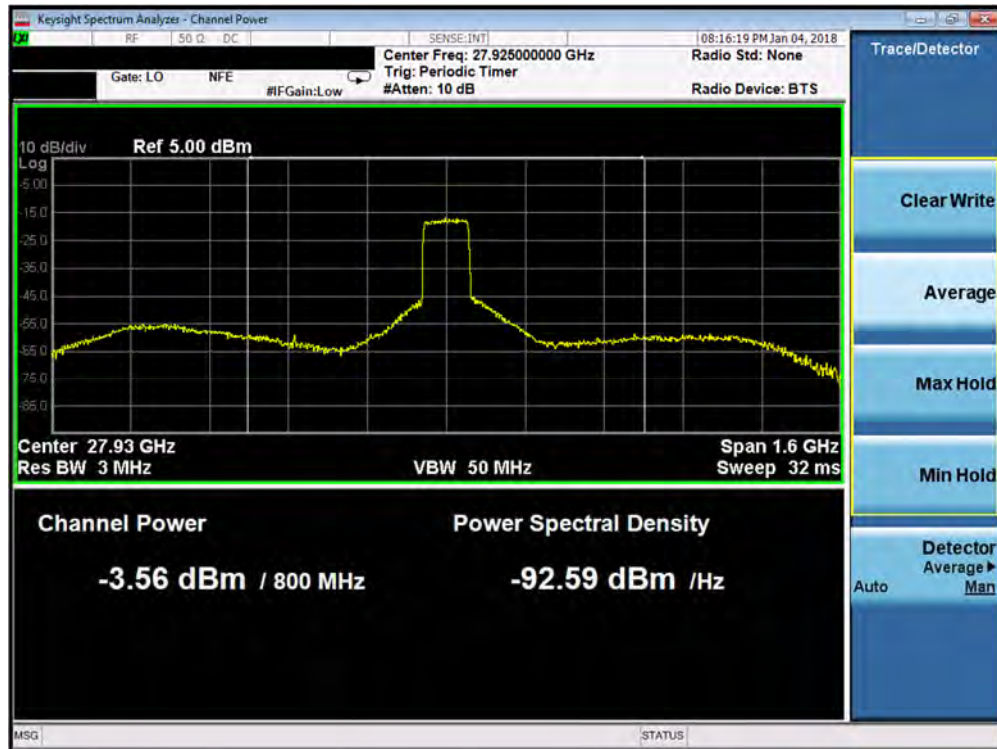
Plot 7-120. Antenna B EIRP Plot (1CC 64QAM Mid Channel)
