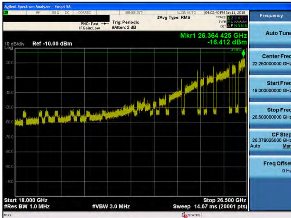
Plot 7-204. Radiated Spurious Plot 18-26.5 GHz (8CC QPSK High Channel, Ant. Angle 45)
