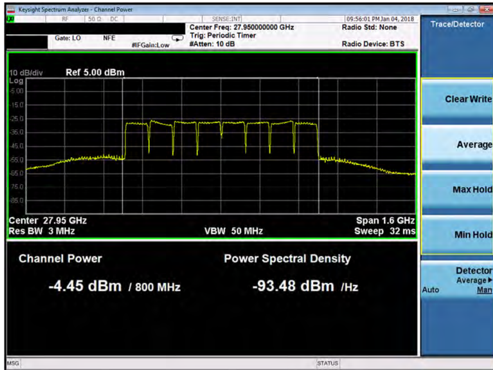
Plot 7-130. Antenna B EIRP Plot (8CC QPSK High Channel)
