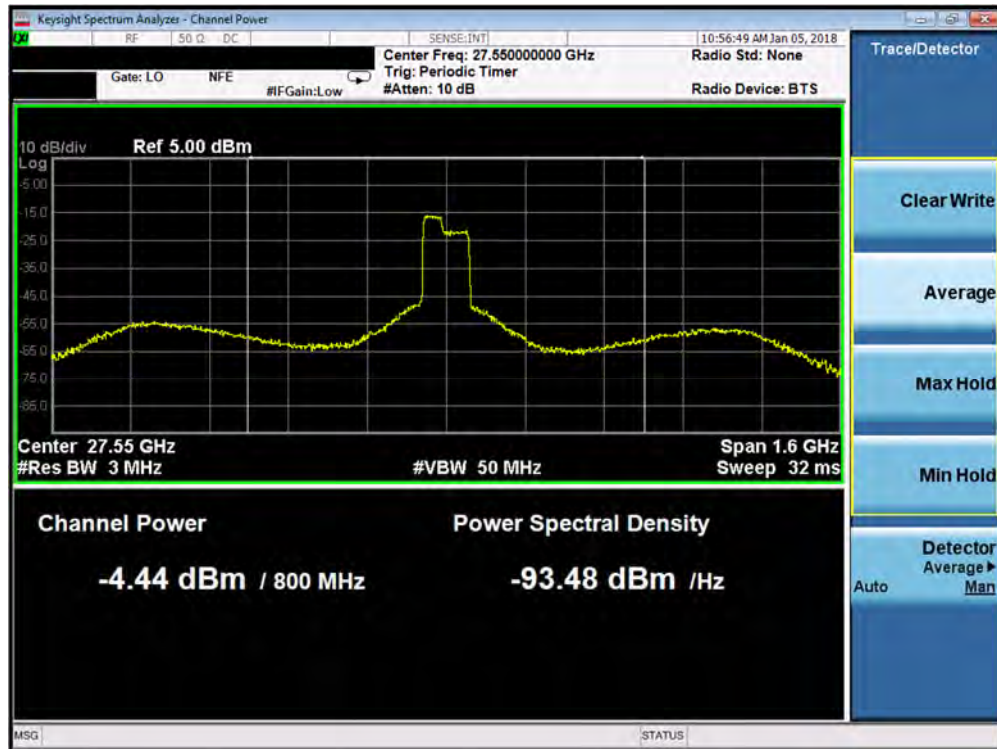
Plot 7-152. Antenna D EIRP Plot (1CC 16QAM Low Channel)
