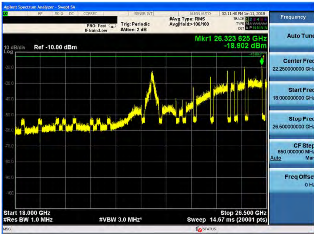
Plot 7-197. Radiated Spurious Plot 18-26.5 GHz (1CC QPSK High Channel, Ant. Angle 135)
