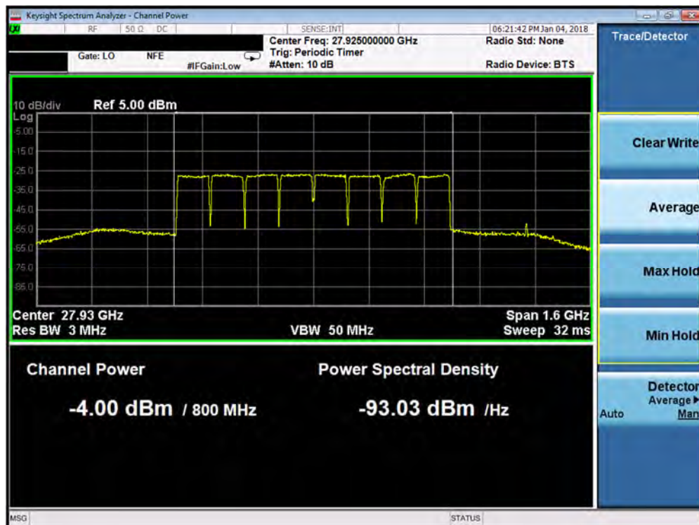
Plot 7-147. Antenna C EIRP Plot (8CC 64QAM Mid Channel)
