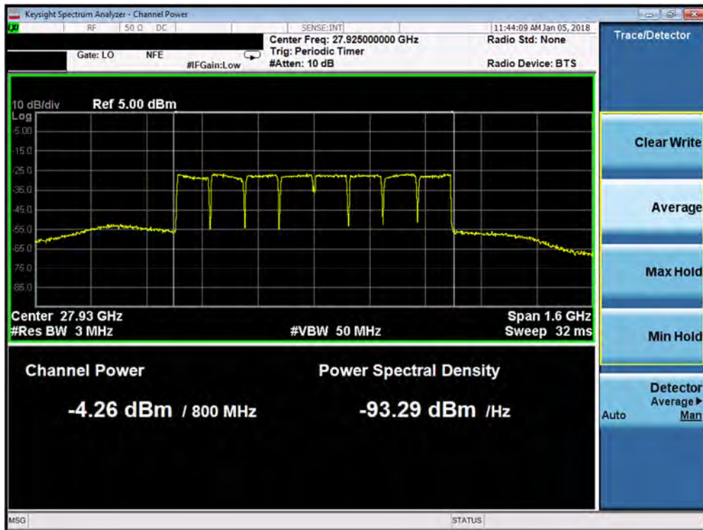
Plot 7-165. Antenna D EIRP Plot (8CC 64QAM Mid Channel)
