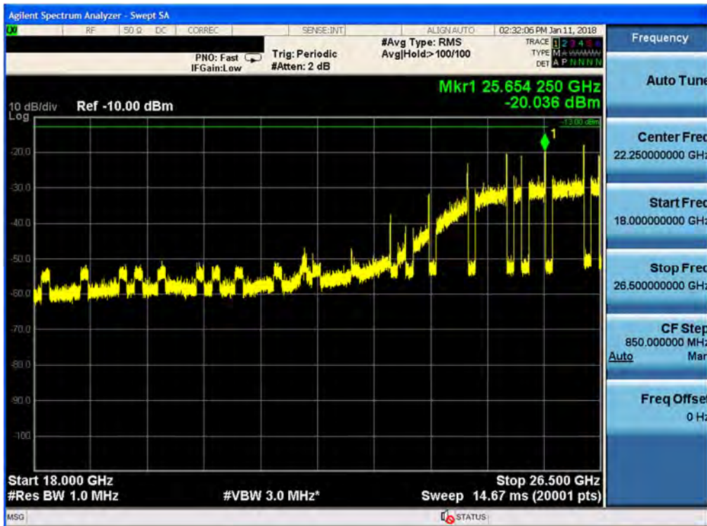
Plot 7-194. Radiated Spurious Plot 18-26.5 GHz (1CC QPSK Low Channel, Ant. Angle 45)
