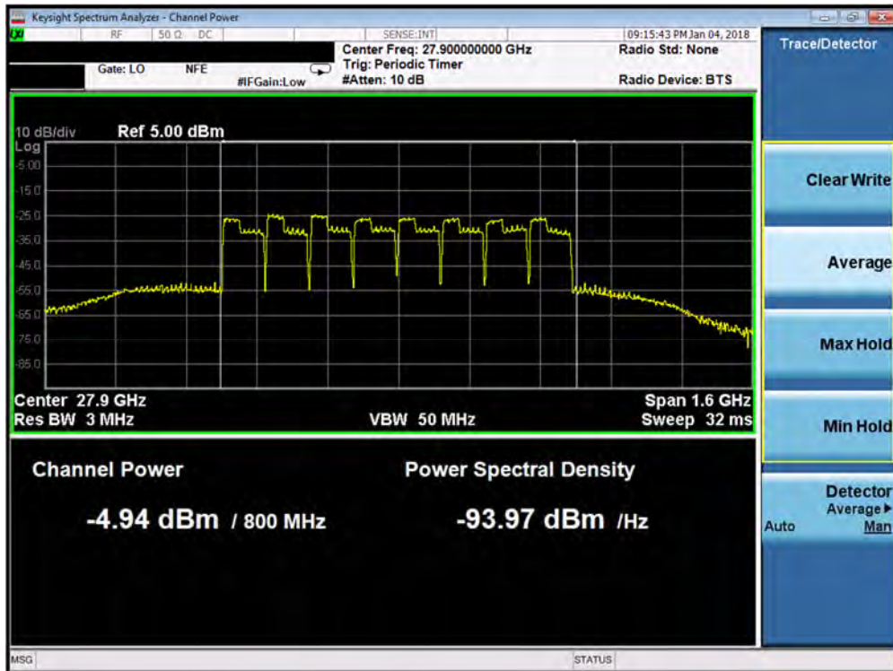
Plot 7-125. Antenna B EIRP Plot (8CC 16QAM Low Channel)
