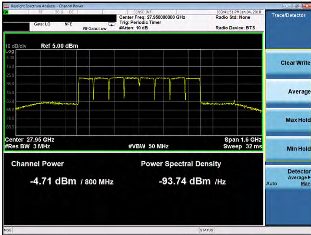
Plot 7-148. Antenna C EIRP Plot (8CC QPSK High Channel)
