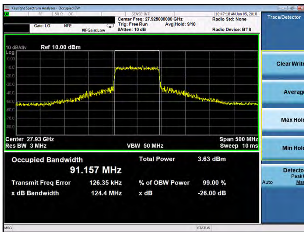
Plot 7-19. Occupied Bandwidth Plot (1CC QPSK Mid Channel)
