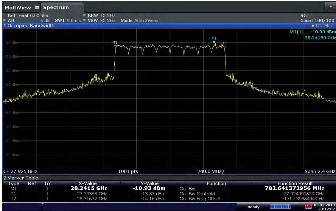
Plot 7-16. Occupied Bandwidth Plot (8CC QPSK Mid Channel)
