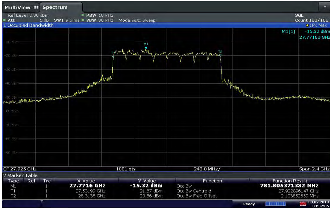
Plot 7-10. Occupied Bandwidth Plot (8CC QPSK Mid Channel)
