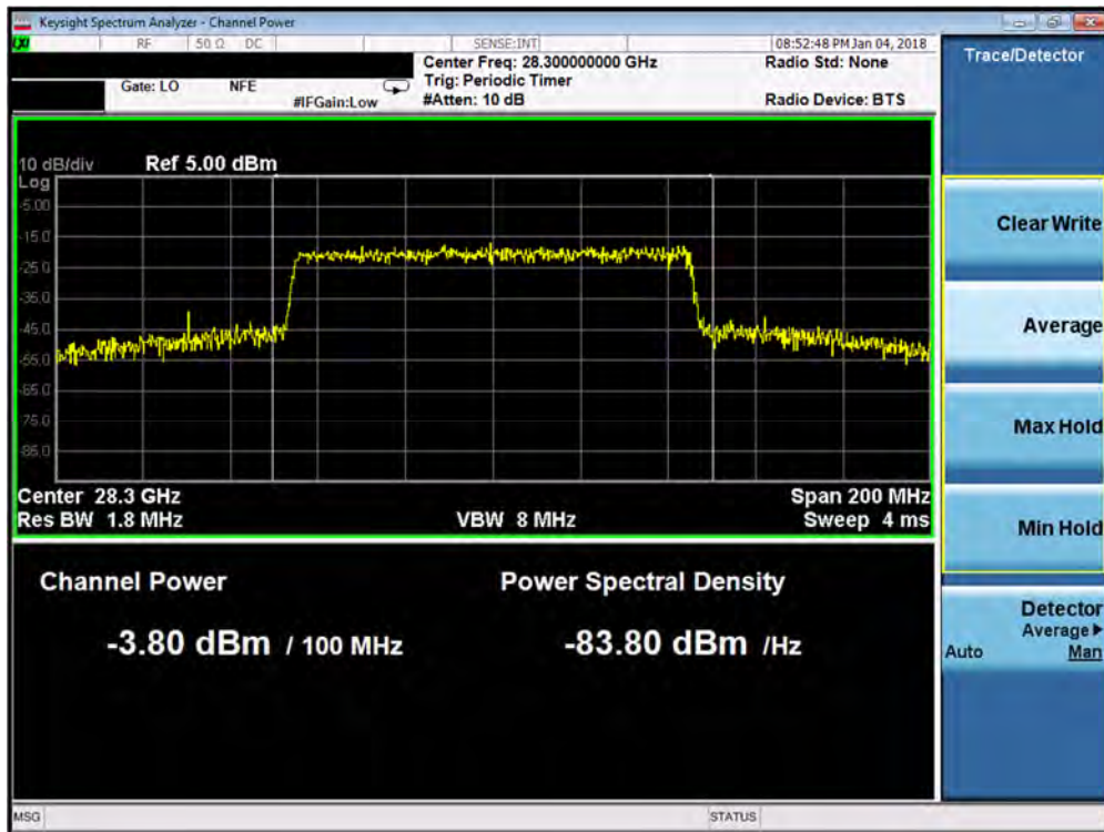
Plot 7-51. Antenna B EIRP Density Plot (1CC 64QAM High Channel)
