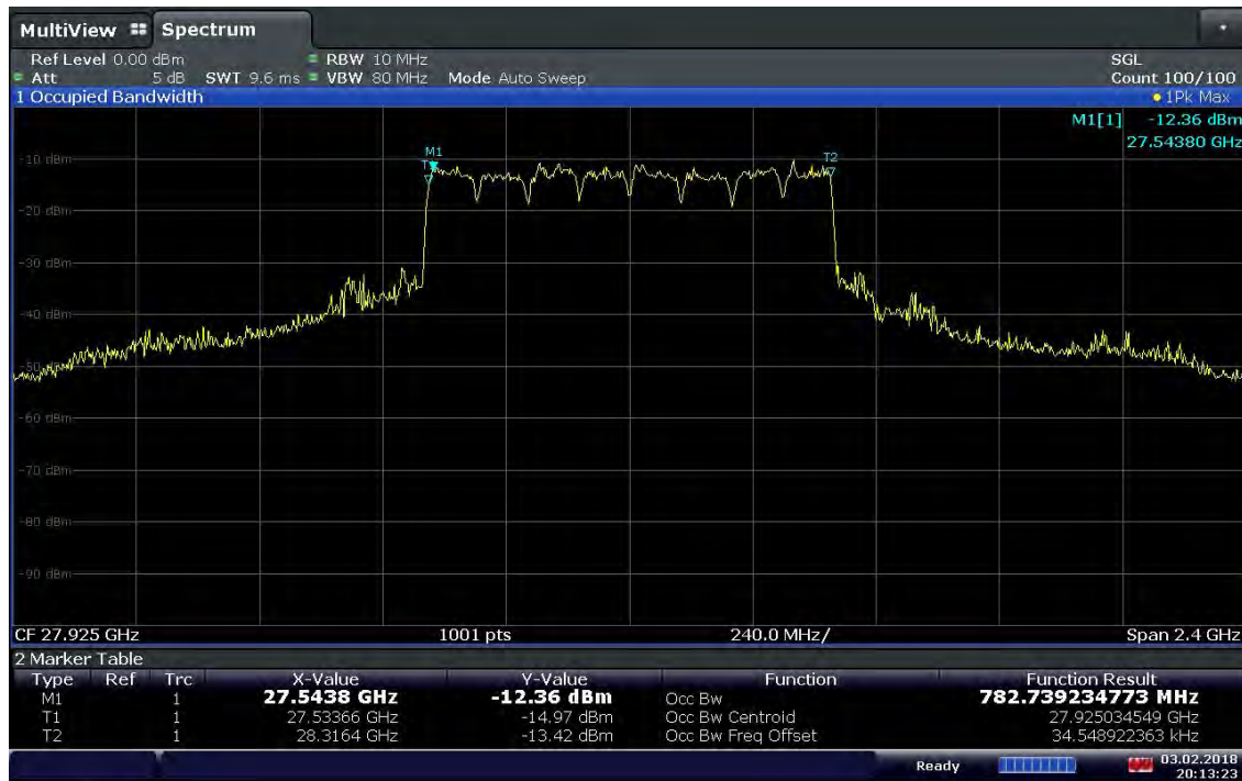
Plot 7-18. Occupied Bandwidth Plot (8CC 64QAM Mid Channel)
