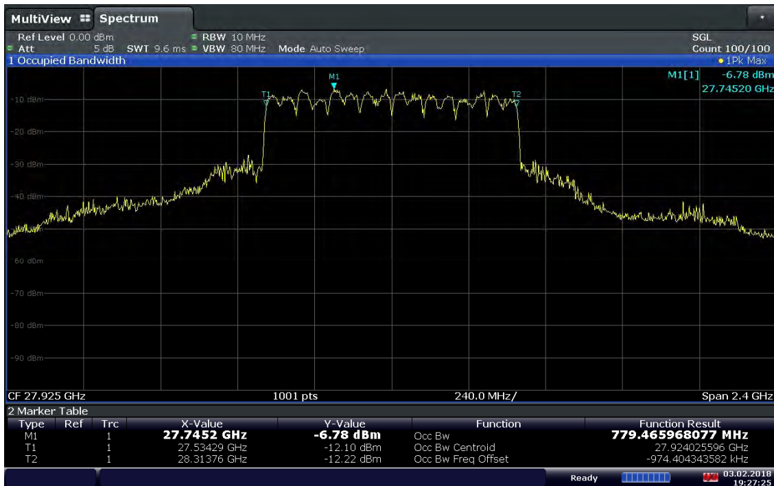
Plot 7-5. Occupied Bandwidth Plot (8CC 16QAM Mid Channel)
