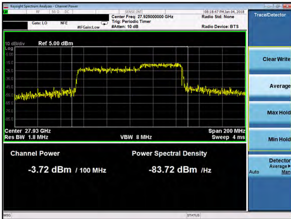
Plot 7-47. Antenna B EIRP Density Plot (1CC 16QAM Mid Channel)
