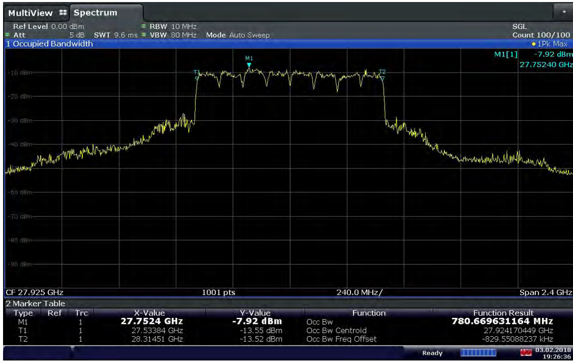
Plot 7-4. Occupied Bandwidth Plot (8CC QPSK Mid Channel)
