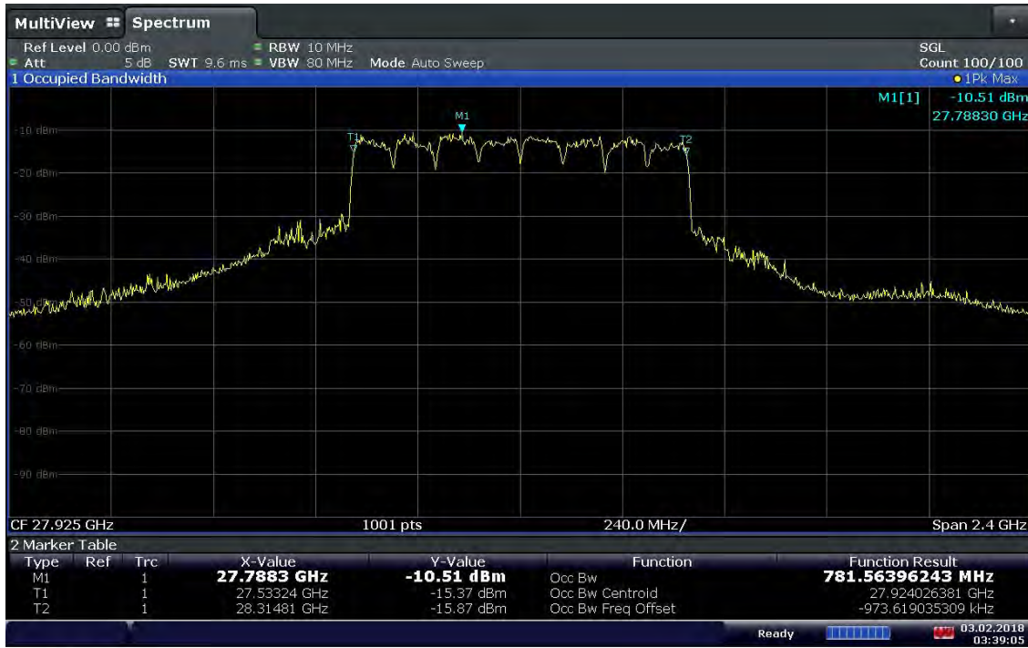
Plot 7-24. Occupied Bandwidth Plot (8CC 64QAM Mid Channel)
