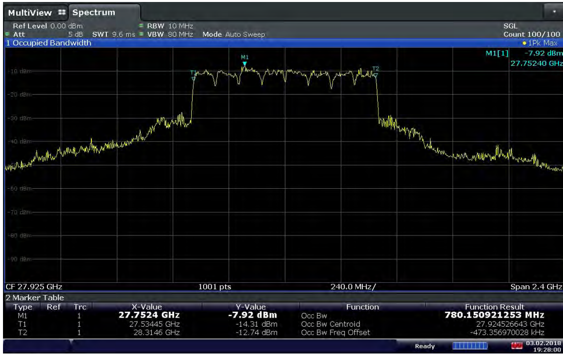
Plot 7-6. Occupied Bandwidth Plot (8CC 64QAM Mid Channel)
