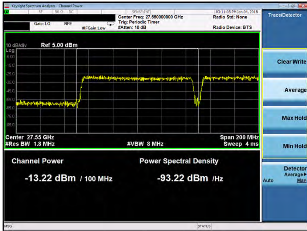
Plot 7-70. Antenna C EIRP Density Plot (8CC QPSK Low Channel)
