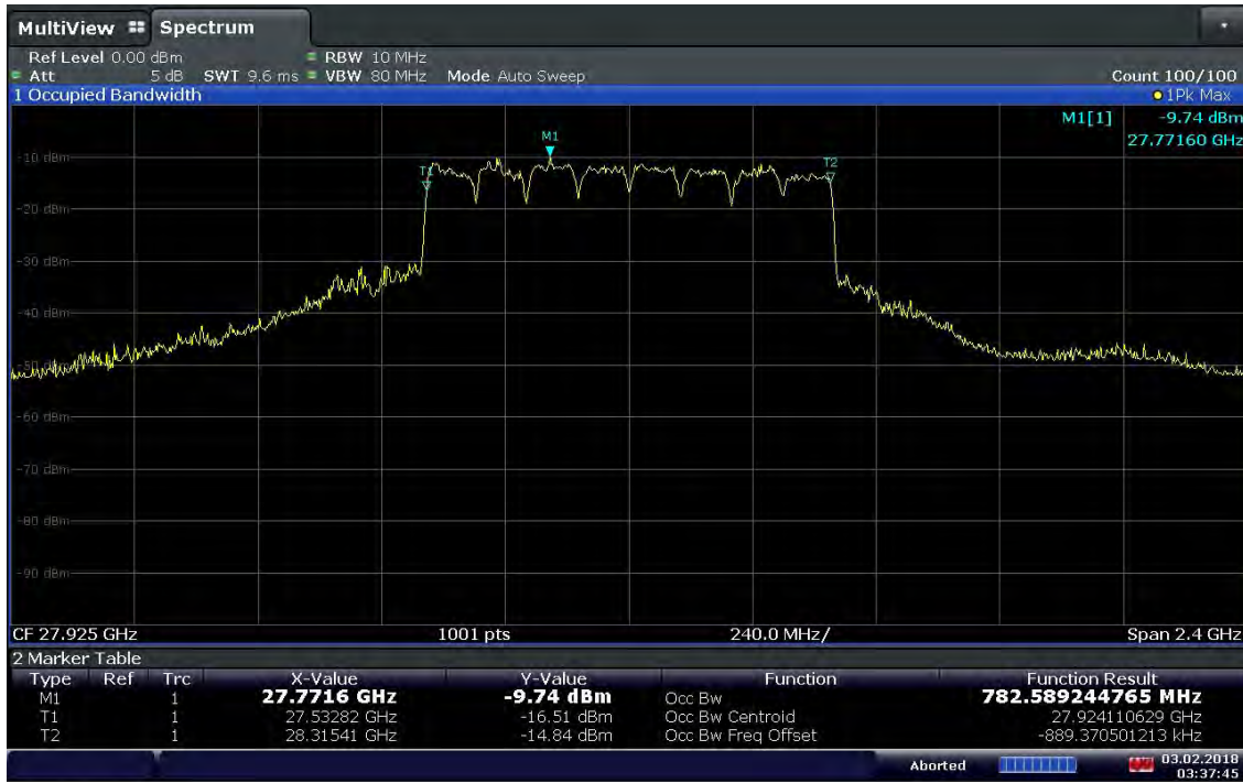
Plot 7-22. Occupied Bandwidth Plot (8CC QPSK Mid Channel)
