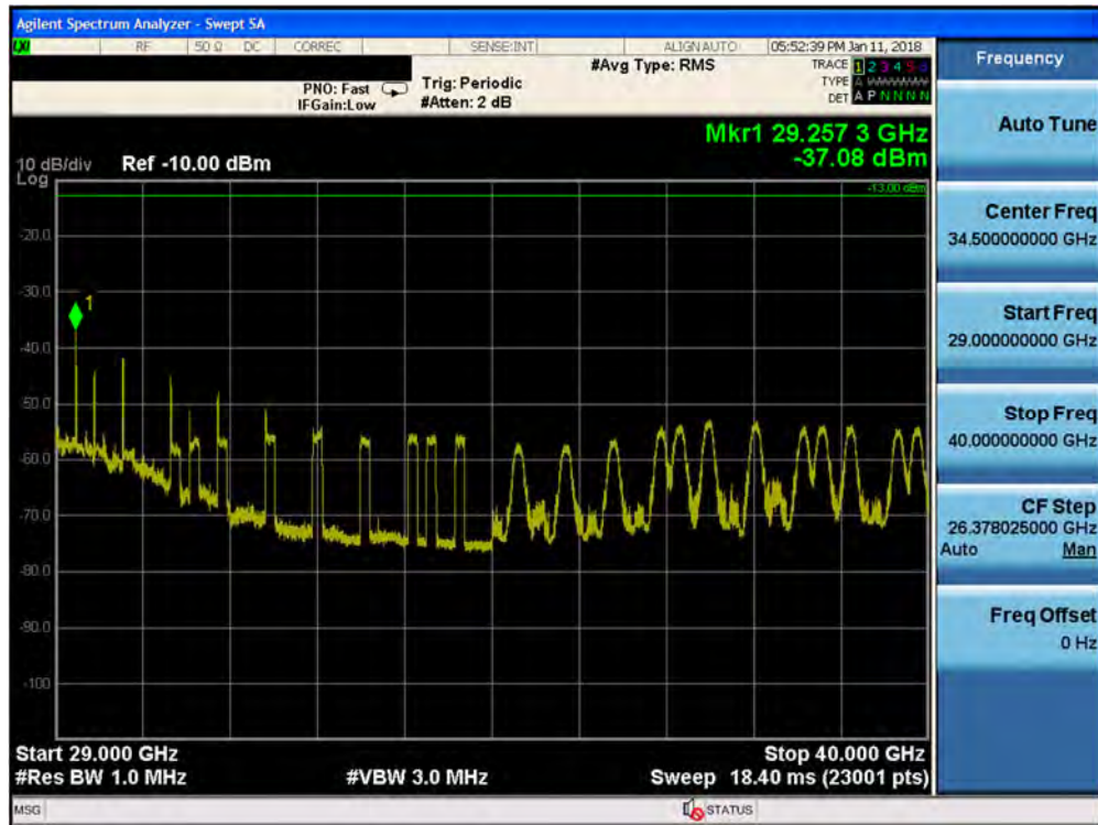
Plot 7-206. Radiated Spurious Plot 26.5-40 GHz (1CC QPSK Low Channel, Ant. Angle 45)
