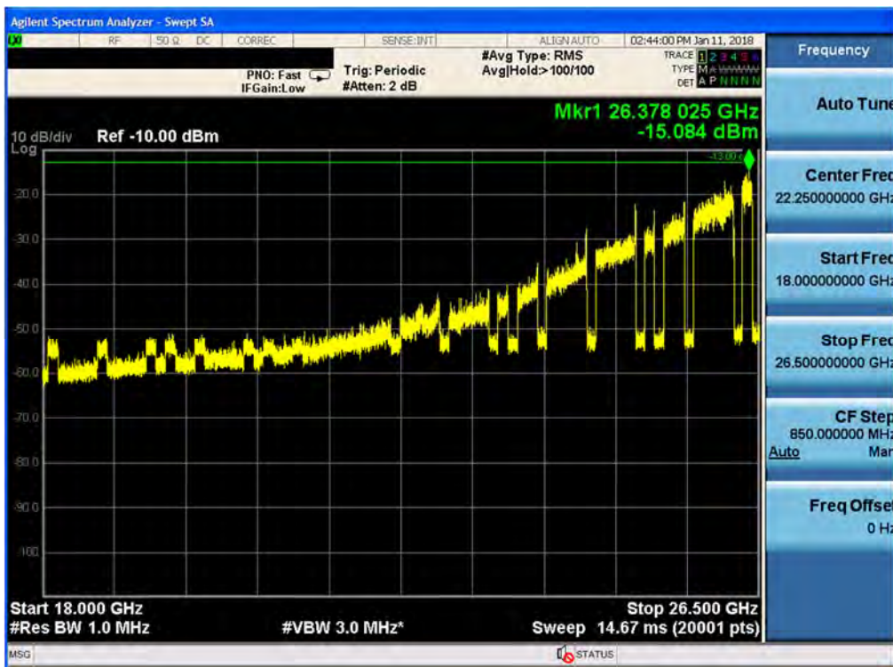
Plot 7-200. Radiated Spurious Plot 18-26.5 GHz (8CC QPSK Low Channel, Ant. Angle 45)
