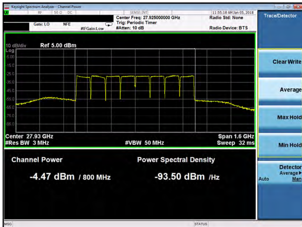
Plot 7-163. Antenna D EIRP Plot (8CC QPSK Mid Channel)
