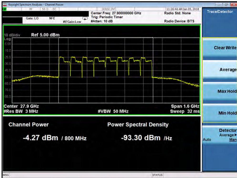
Plot 7-161. Antenna D EIRP Plot (8CC 16QAM Low Channel)
