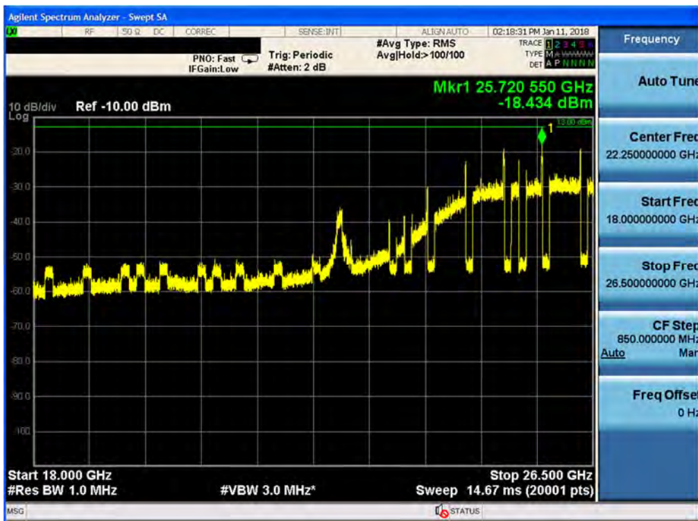
Plot 7-198. Radiated Spurious Plot 18-26.5 GHz (1CC QPSK High Channel, Ant. Angle 45)
