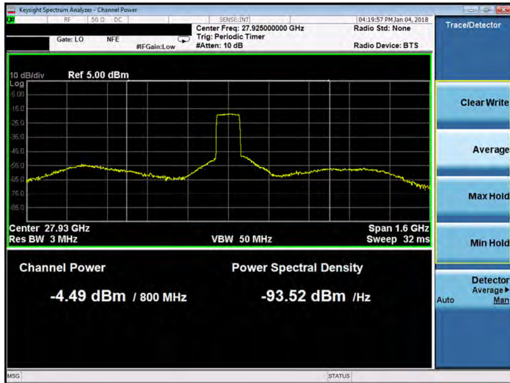
Plot 7-100. Antenna A EIRP Plot (1CC QPSK Mid Channel)
