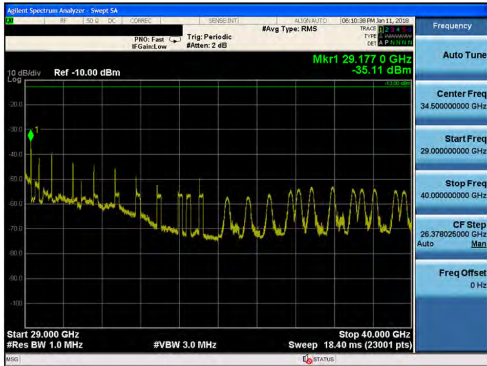
Plot 7-210. Radiated Spurious Plot 26.5-40 GHz (1CC QPSK High Channel, Ant. Angle 45)
