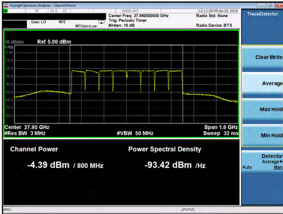
Plot 7-166. Antenna D EIRP Plot (8CC QPSK High Channel)
