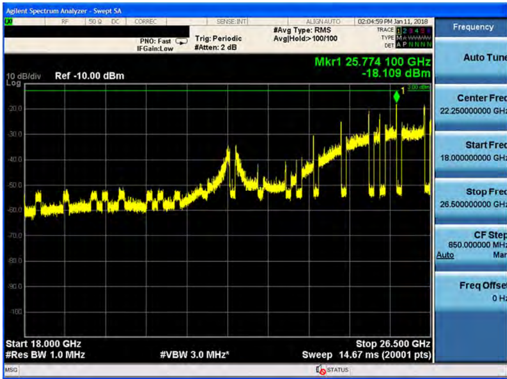
Plot 7-195. Radiated Spurious Plot 18-26.5 GHz (1CC QPSK Mid Channel, Ant. Angle 135)
