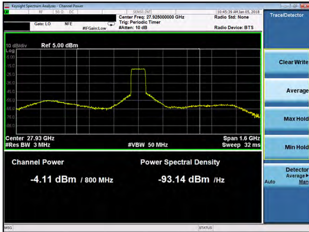
Plot 7-154. Antenna D EIRP Plot (1CC QPSK Mid Channel)
