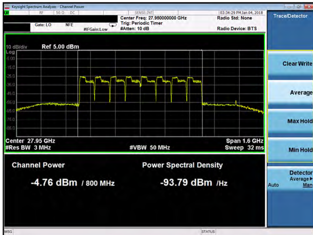
Plot 7-149. Antenna C EIRP Plot (8CC 16QAM High Channel)
