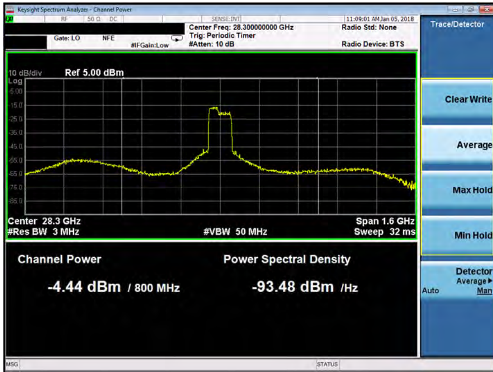
Plot 7-158. Antenna D EIRP Plot (1CC 16QAM High Channel)
