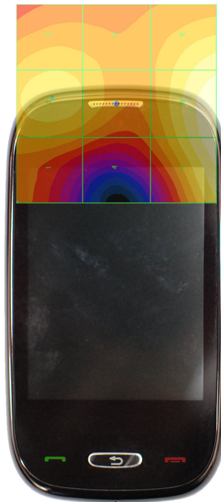
Figure 18-4 E-Field WD Scan overlay
