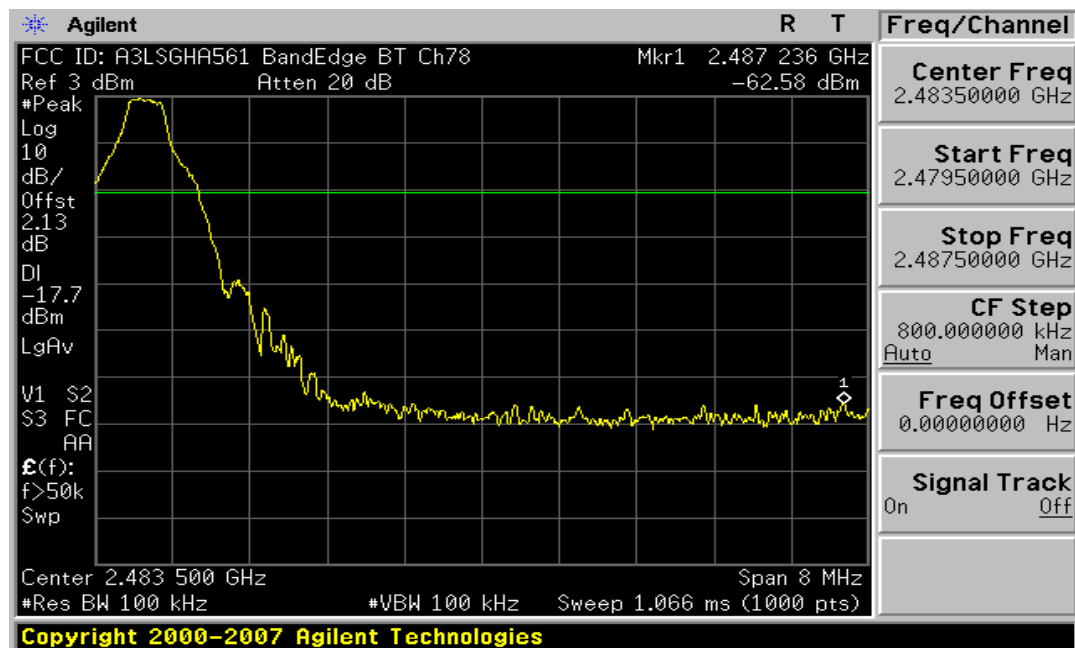
Plot 6-5. Band Edge Plot (Bluetooth – Ch. 78)
