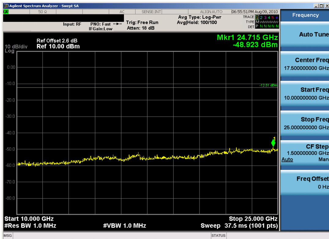
Plot 6-17. Conducted Spurious Plot (Bluetooth – Ch. 78)
