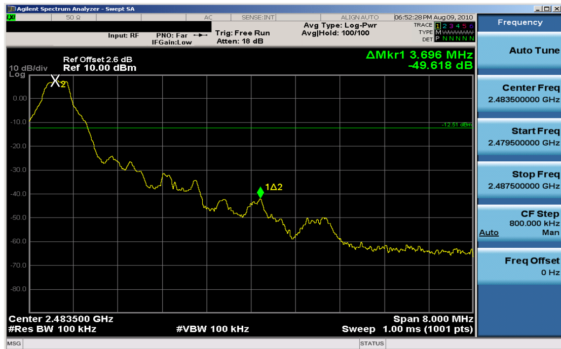
Plot 6-5. Band Edge Plot (Bluetooth – Ch. 78)
