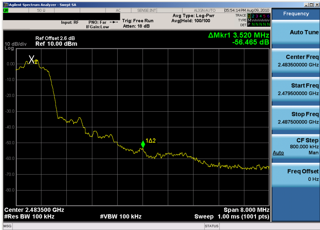
Plot 6-7. Band Edge Plot (Bluetooth (EDR) - Ch. 78)
