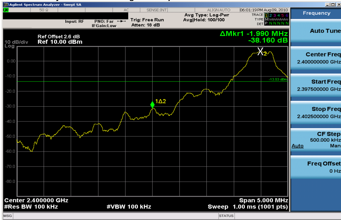
Plot 6-4. Band Edge Plot (Bluetooth – Ch. 0)
