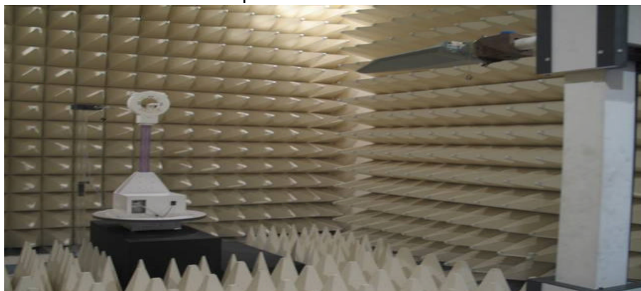
Figure2. Photograph of 3m Fully-Anechoic Chamber
