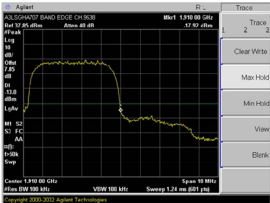
Plot A-18. Band Edge Plot (PCS WCDMA Mode – Ch. 9538)
