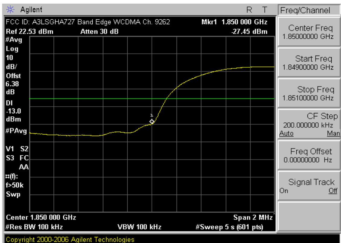
Plot 7-34. Band Edge Plot (PCS WCDMA Mode – Ch. 9262)
