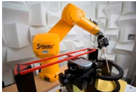
Figure 5-5 SPEAG Robotic System
