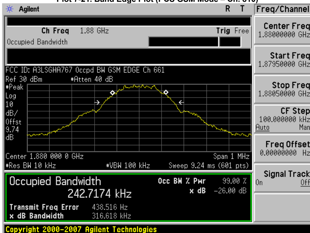
Plot 7-22. Occupied Bandwidth Plot (EDGE1900 Mode – Ch. 661)
