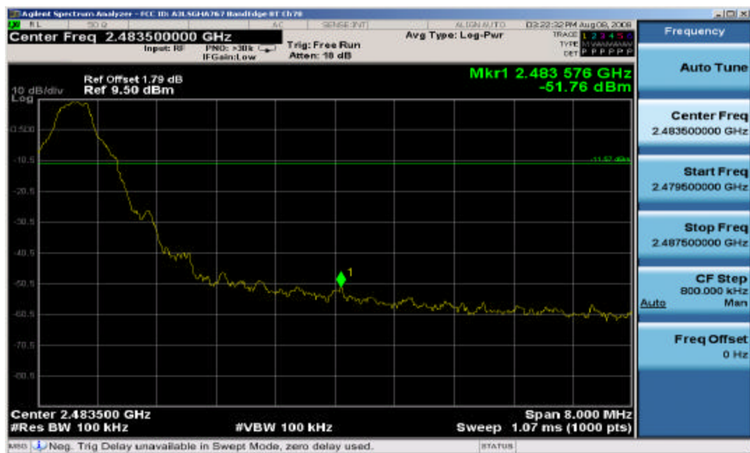
Plot 6-5. Band Edge Plot (Bluetooth – Ch. 78)
