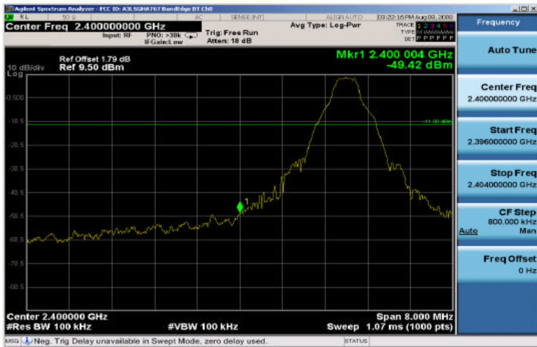
Plot 6-4. Band Edge Plot (Bluetooth – Ch. 0)
