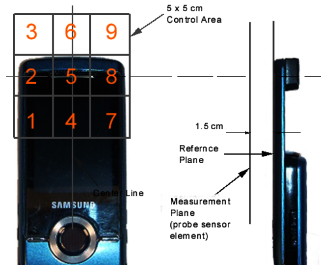
Figure 17-3 5x5 Scan grid above WD
