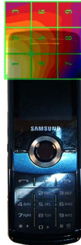
Figure 17-5 H-Field WD Scan overlay
