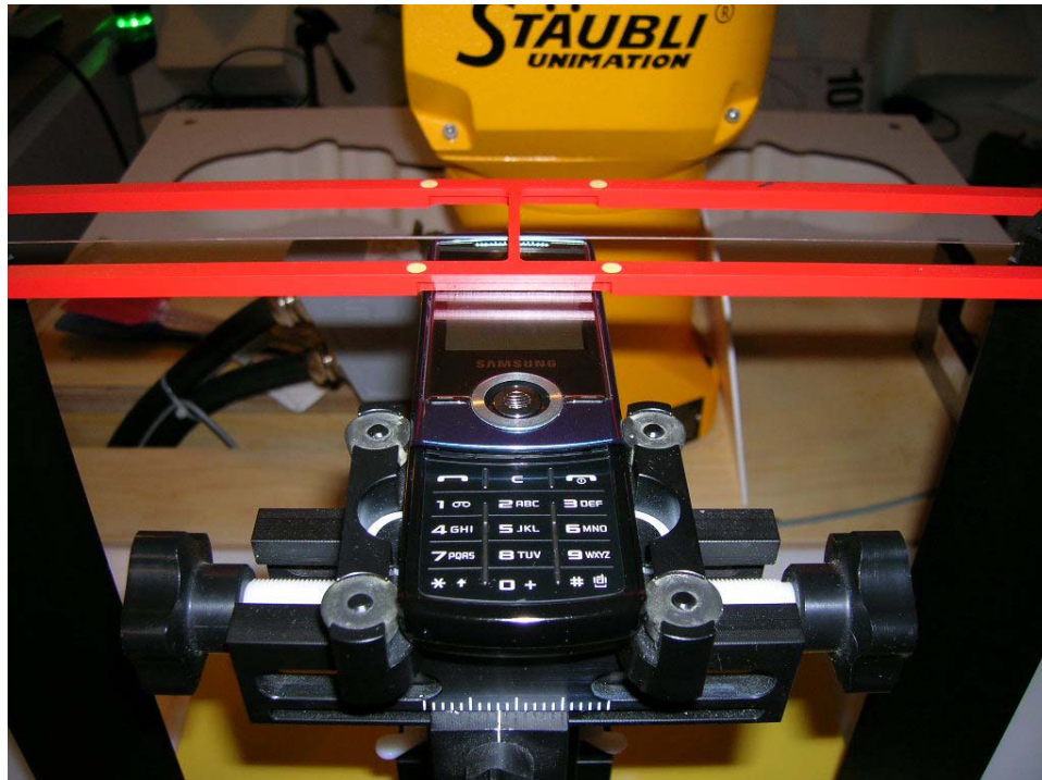
Figure 17-1 Ear Reference Point HAC Phantom Alignment
