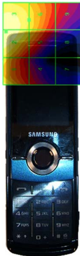
Figure 17-4 E-Field WD Scan overlay
