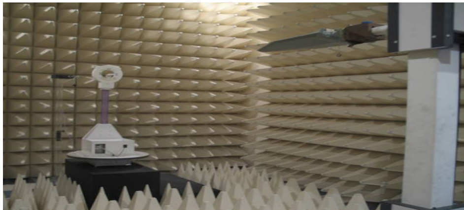
Figure2. Photograph of 3m Fully-Anechoic Chamber
