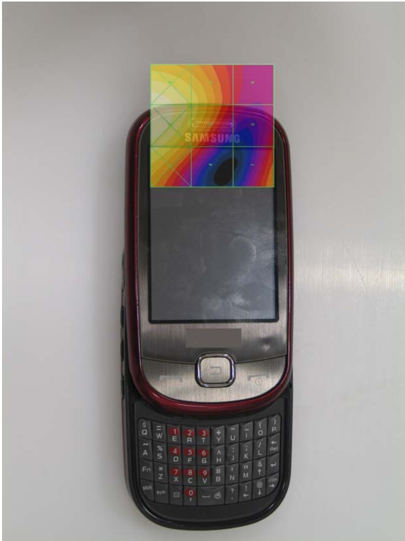
Scan overlay with actual device (E-field)
