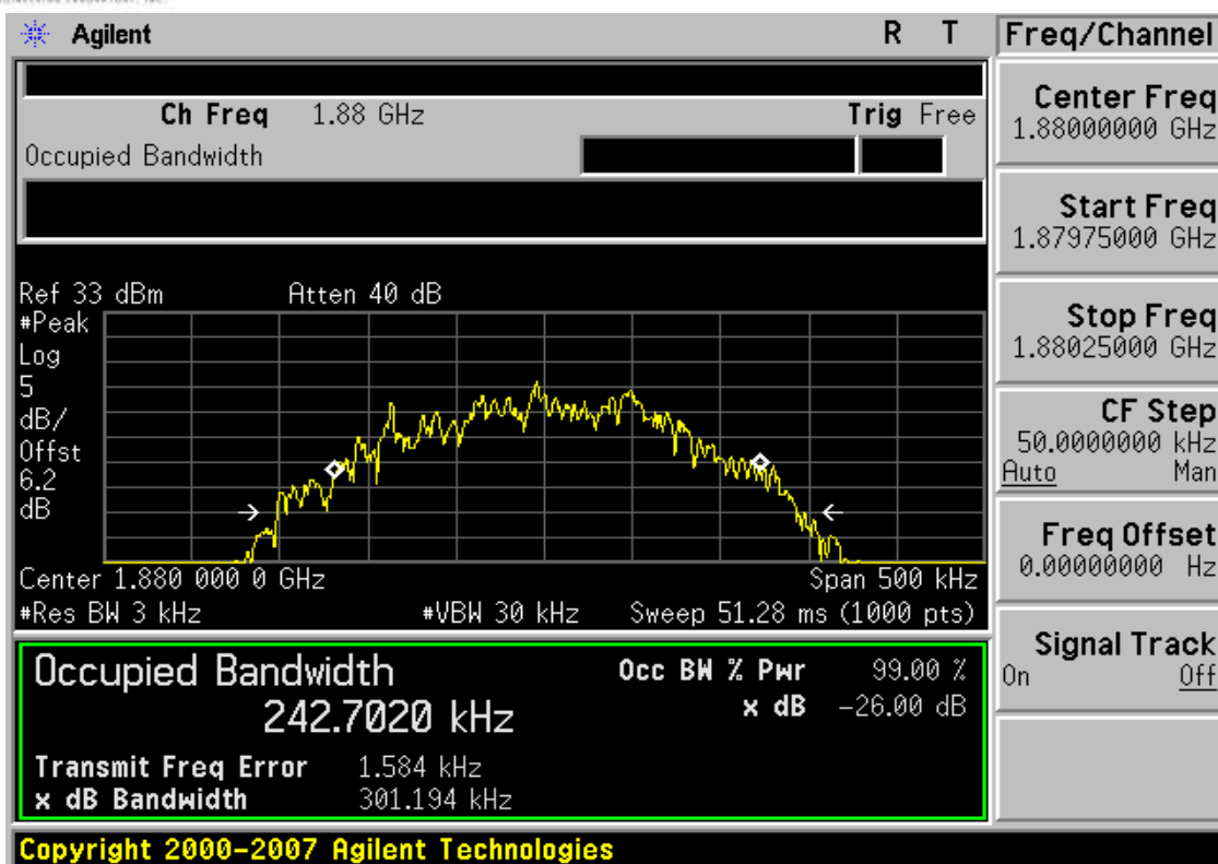
Plot 7-21. Occupied Bandwidth Plot (EDGE1900 Mode – Ch. 661)
