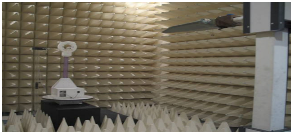
Figure2. Photograph of 3m Fully-Anechoic Chamber
