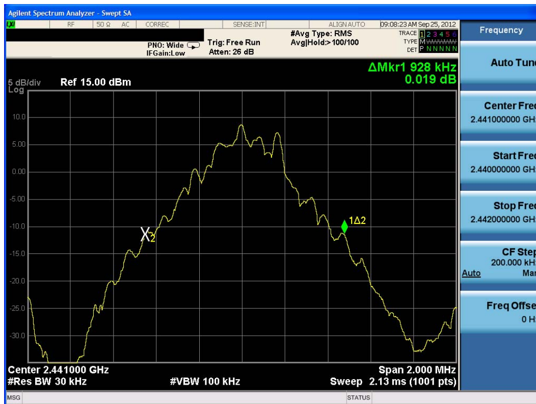
Plot 6-2. 20dB Bandwidth Plot (Bluetooth, 1Mbps - Ch. 39)
