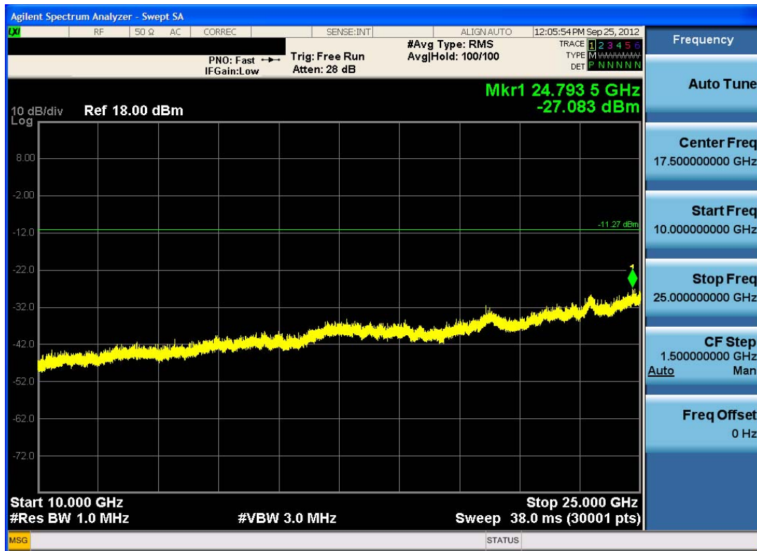
Plot 6-32. Conducted Spurious Plot (Bluetooth, 1Mbps – Ch. 78)
