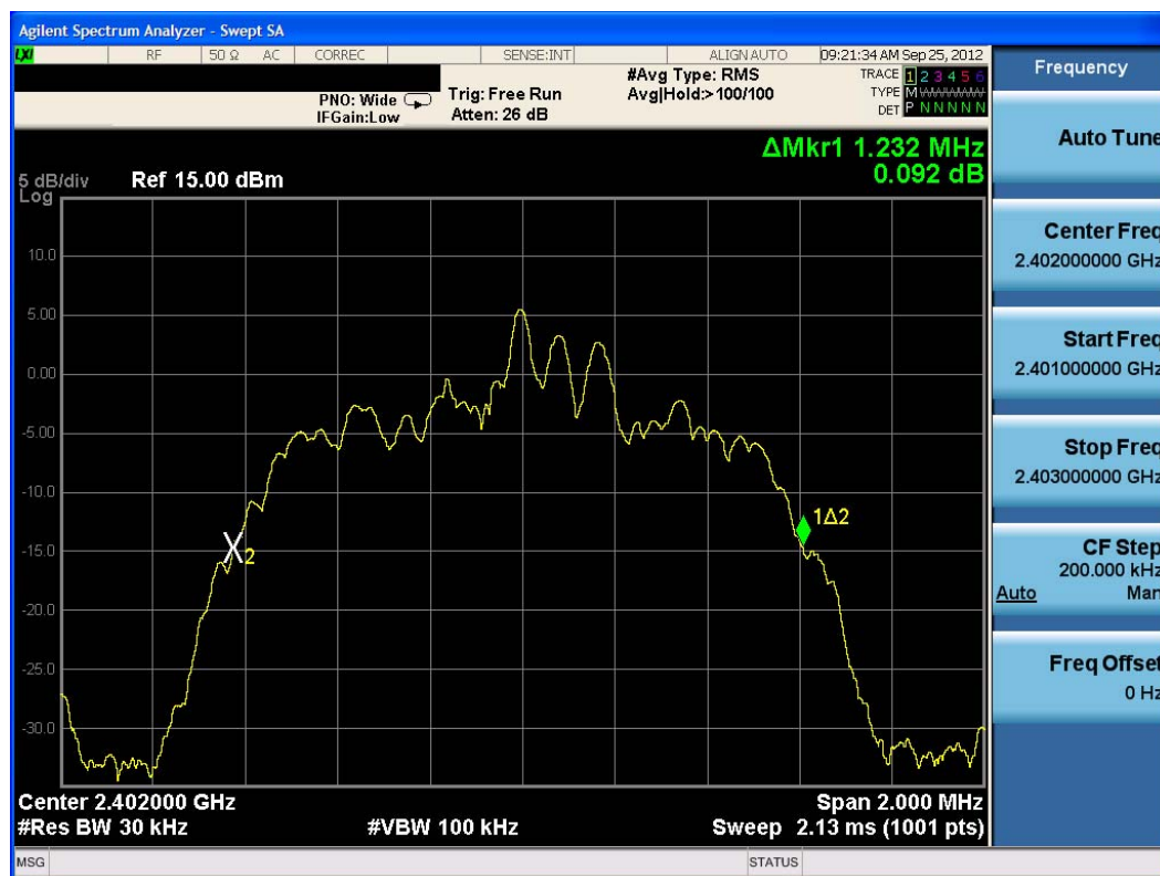
Plot 6-4. 20dB Bandwidth Plot (Bluetooth, 2Mbps – Ch. 0)
