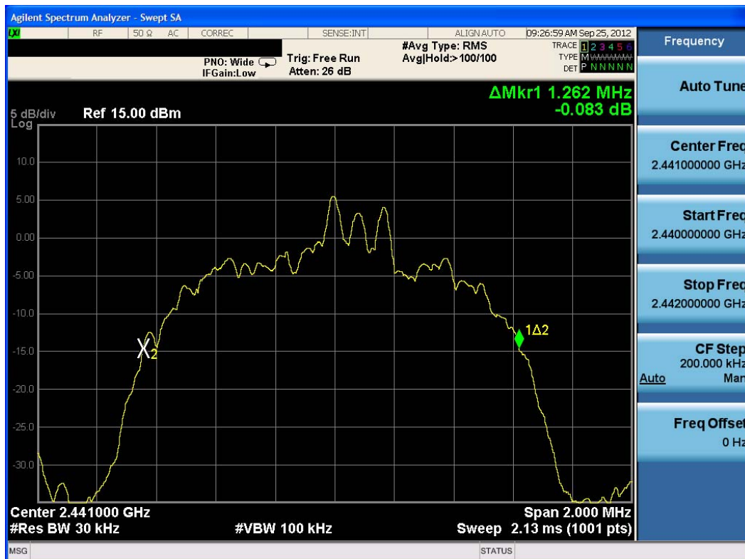
Plot 6-8. 20dB Bandwidth Plot (Bluetooth, 3Mbps – Ch. 39)
