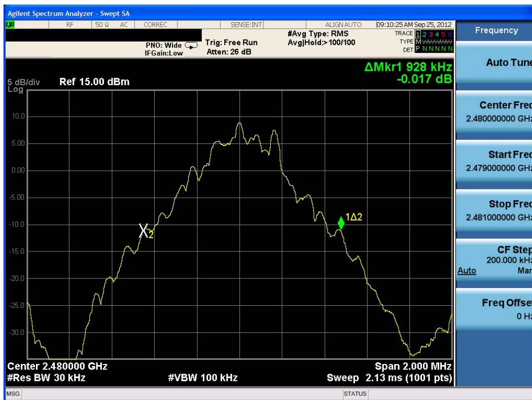
Plot 6-3. 20dB Bandwidth Plot (Bluetooth, 1Mbps – Ch. 78)
