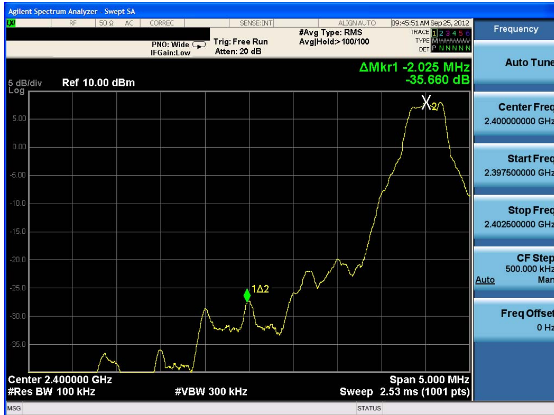
Plot 6-19. Band Edge Plot (Bluetooth with Hopping Disabled, 1Mbps – Ch. 0)
