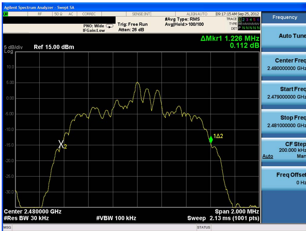
Plot 6-6. 20dB Bandwidth Plot (Bluetooth, 2Mbps – Ch. 78)
