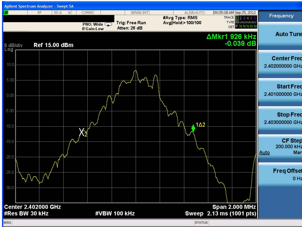
Plot 6-1. 20dB Bandwidth Plot (Bluetooth, 1Mbps - Ch. 0)
