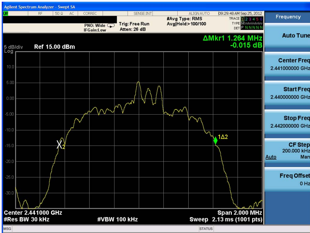
Plot 6-9. 20dB Bandwidth Plot (Bluetooth, 3Mbps – Ch. 78)
