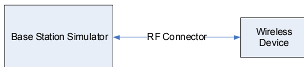
Figure 11-1 Power Measurement Setup
