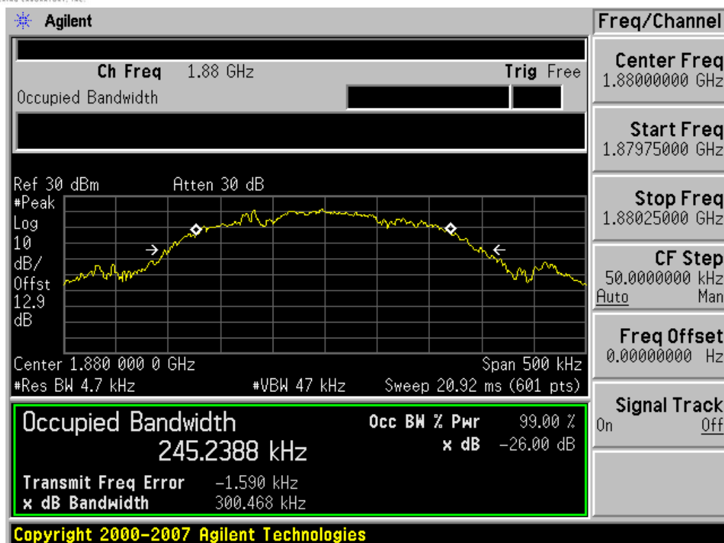
Plot 7-21. Occupied Bandwidth Plot (EDGE1900 Mode – Ch. 661)
