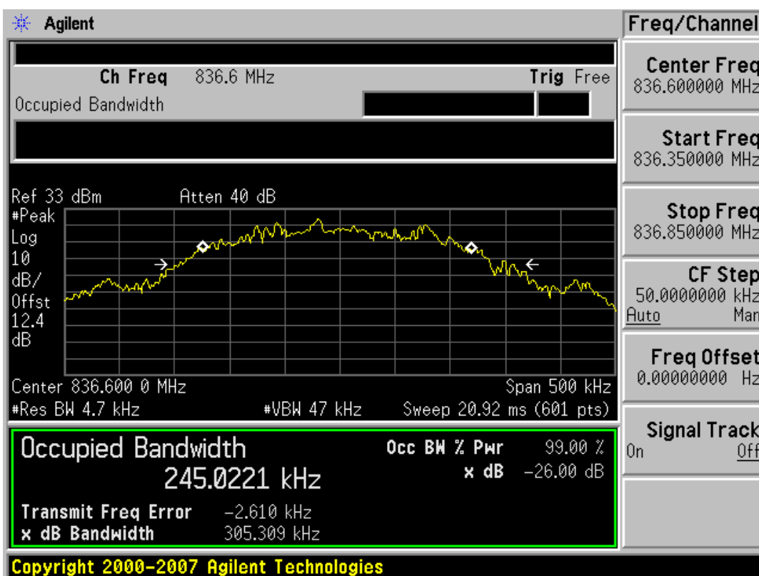
Plot 7-10. Occupied Bandwidth Plot (EDGE850 Mode - Ch. 190)
