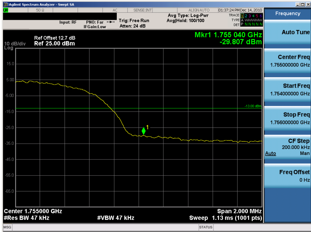
Plot 7-33. Band Edge Plot (AWS WCDMA Mode – Ch. 1862)
