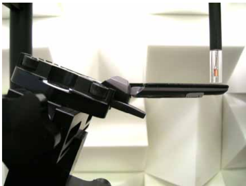
Figure 12-2 Test Setup for Wireless Device
