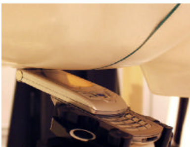
Figure 8.3 Right Head SAR Test Setup -- Ear/Tilt 15° Position--
