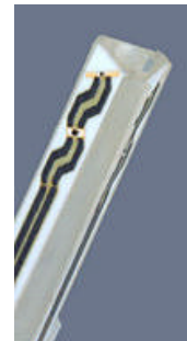
Figure 3.4 Probe Thick-Film Technique
