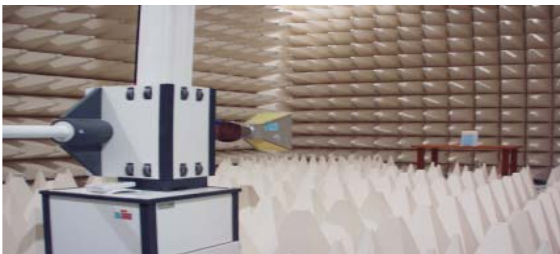
Figure2. Photograph of 3m Fully Anechoic Chamber
