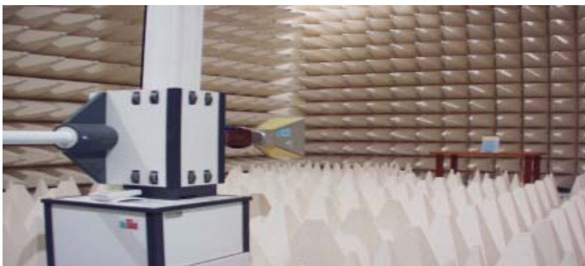
Figure2. Photograph of 3m Fully Anechoic Chamber
