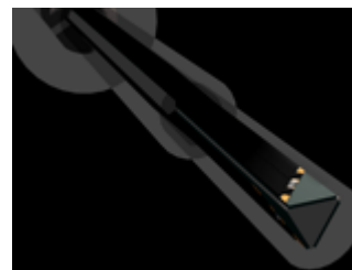
Figure 4-3 Triangular Probe Configuration
