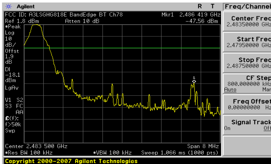
Plot 6-5. Band Edge Plot (Bluetooth – Ch. 78)
