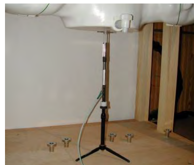
Figure 10-2 System Verification Setup Photo
