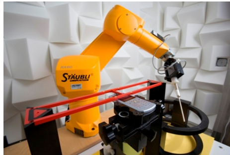
Figure 5-3 SPEAG Robotic System
