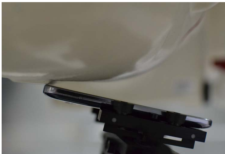
SAR Test Setup Photo 2 – Right Tilt
