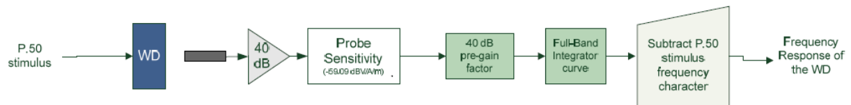
Figure 5-13 Frequency Response Block Diagram
