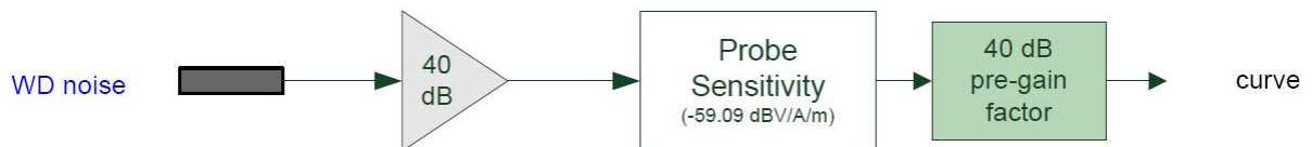
Figure 6-2 Audio Band Magnetic Curve Measurement Block Diagram
