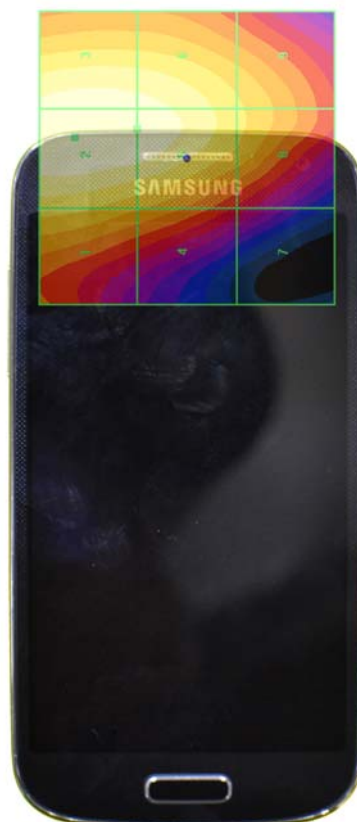
Figure 18-4 E-Field WD Scan overlay
