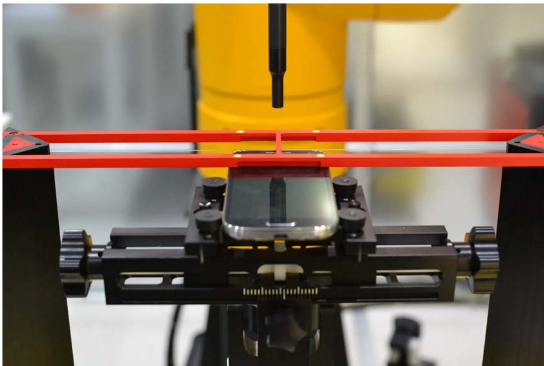
Figure 18-1 Ear Reference Point HAC Phantom Alignment
