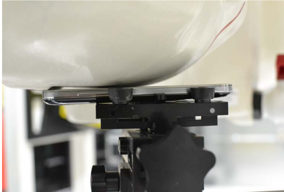
SAR Test Setup Photo 1: Right Cheek
