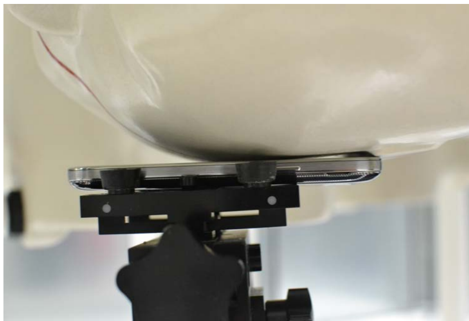
SAR Test Setup Photo 3: Left Cheek
