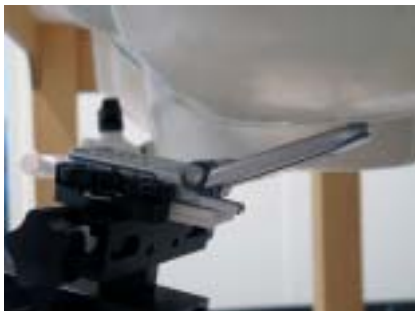
Figure 8.5 Left Head SAR Test Setup -- Ear/Tilt 15° Position--
