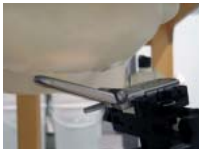
Figure 8.3 Right Head SAR Test Setup -- Ear/Tilt 15° Position--
