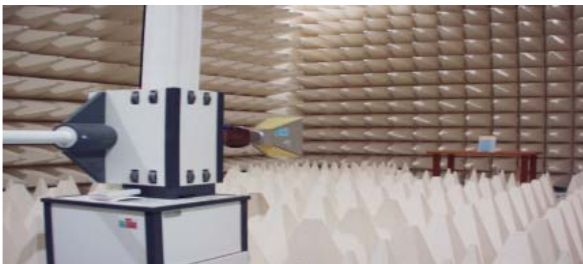
Figure2. Photograph of 3m Fully Anechoic Chamber
