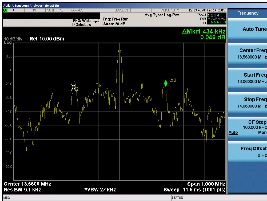
Figure 8-2. 20dB Bandwidth Plot
