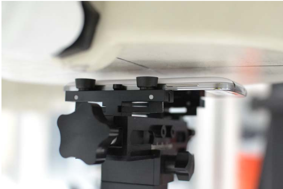
SAR Test Setup Photo 7: Back at 1.0 cm with Wireless Charging Cover
